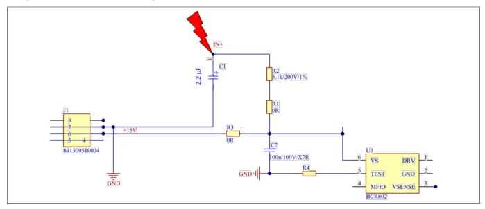
Figure 16 Access point of ESD gun test - schematic
