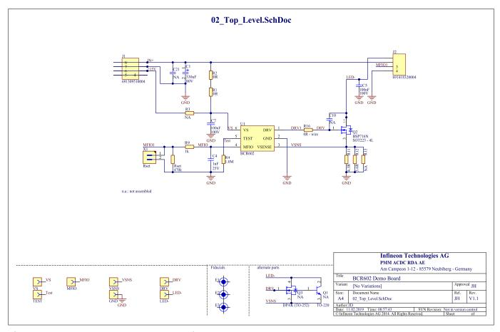
Figure 4 BCR602 PCB schematics
