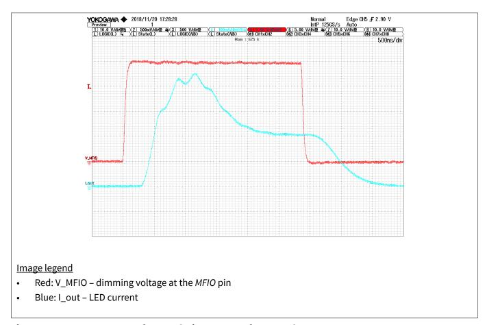
Figure 13 PWM-on reference design MOSFET,  $f_{PWM} = 3.5 \text{ kHz}$
