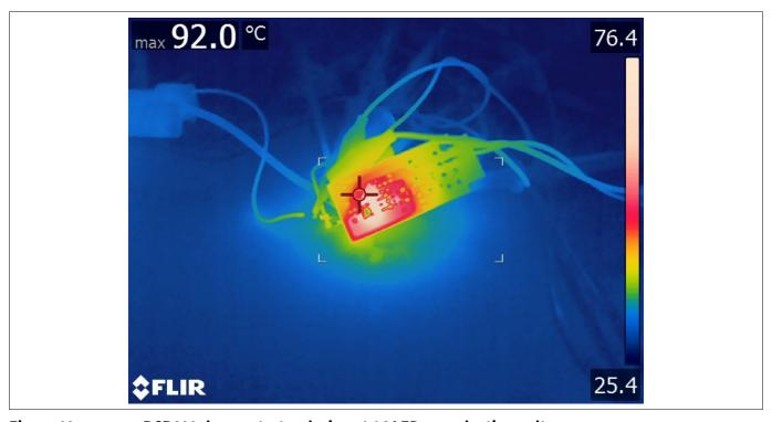
Figure 19 BCR602 demonstrator design at 14 LEDs, production voltage
