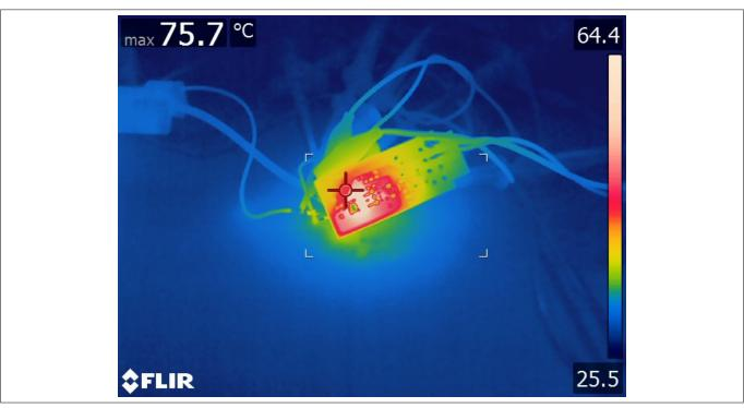
Figure 20 BCR602 demonstrator design at 14 LEDs, 6 V AC ripple, 41 V DC voltage
