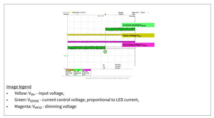
Figure 15 OTP deactivation at 116°C, 15 LEDs
