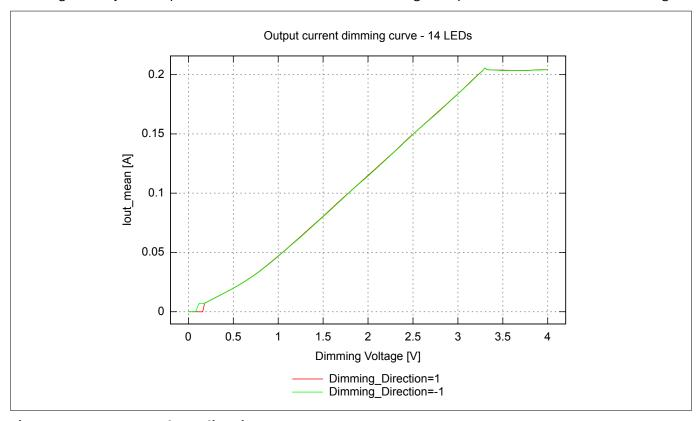
DC voltage dimming curve Figure 9
