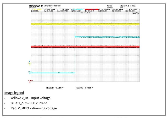
Figure 14 Hot-plug at three LEDs, 200 mA target current, power MOSFET
