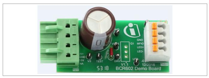
Figure 2 Top side of the demonstrator design board (56.00 mm x 27.00 mm)
