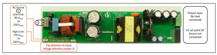
Figure 4 No-load system standby power test setup
