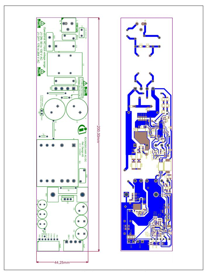
Figure 7 PCB top (left) and bottom (right) layout of the reference design board
