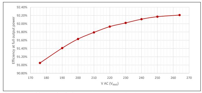
Figure 9 Efficiency at high-line input and full output power (84 W)
