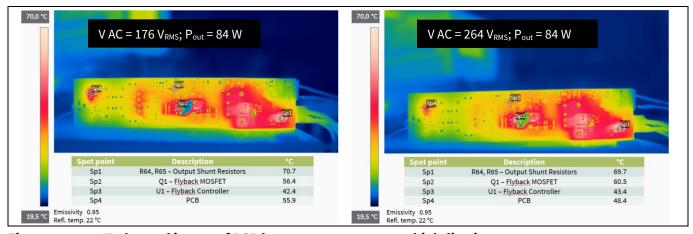
Figure 12 IR thermal image of PCB bottom components at high-line input
