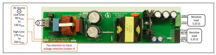
Figure 3 EMI test setup with full output power
