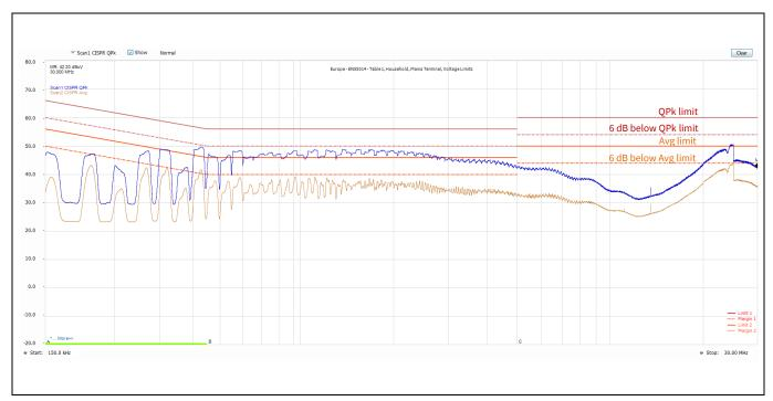
Figure 16 Conducted emissions (live) test result at VAC = 110  $V_{RMS}$ ,  $F_{line}$  = 50 Hz,  $P_{out}$  = 84 W
