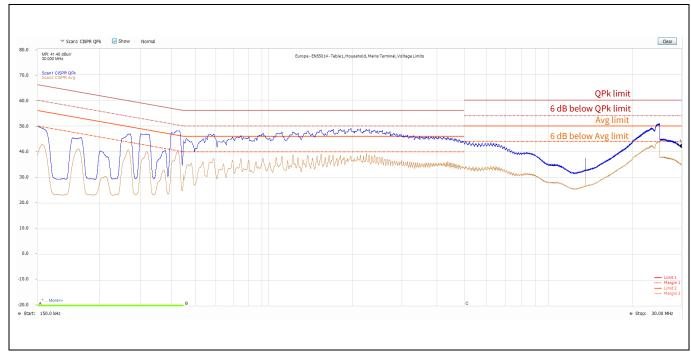
Figure 17 Conducted emissions (neutral) test result at V AC = 110  $V_{RMS}$ ,  $F_{line}$  = 50 Hz,  $P_{out}$  = 84 W
