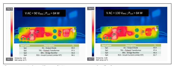
Figure 15 IR thermal image of PCB top components at low-line input
