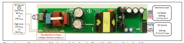
Figure 2 Test setup with electronic load and adjustable CC set-point using DC source
