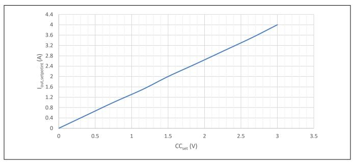
For power tool battery charger with 110 V AC / 230 V AC rated input and constant current (CC) output up to 4 A
