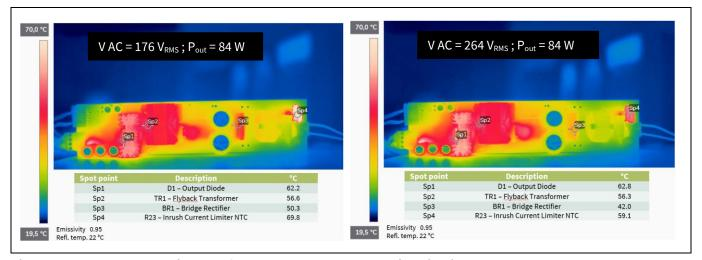
IR thermal image of PCB top components at high-line input Figure 13
