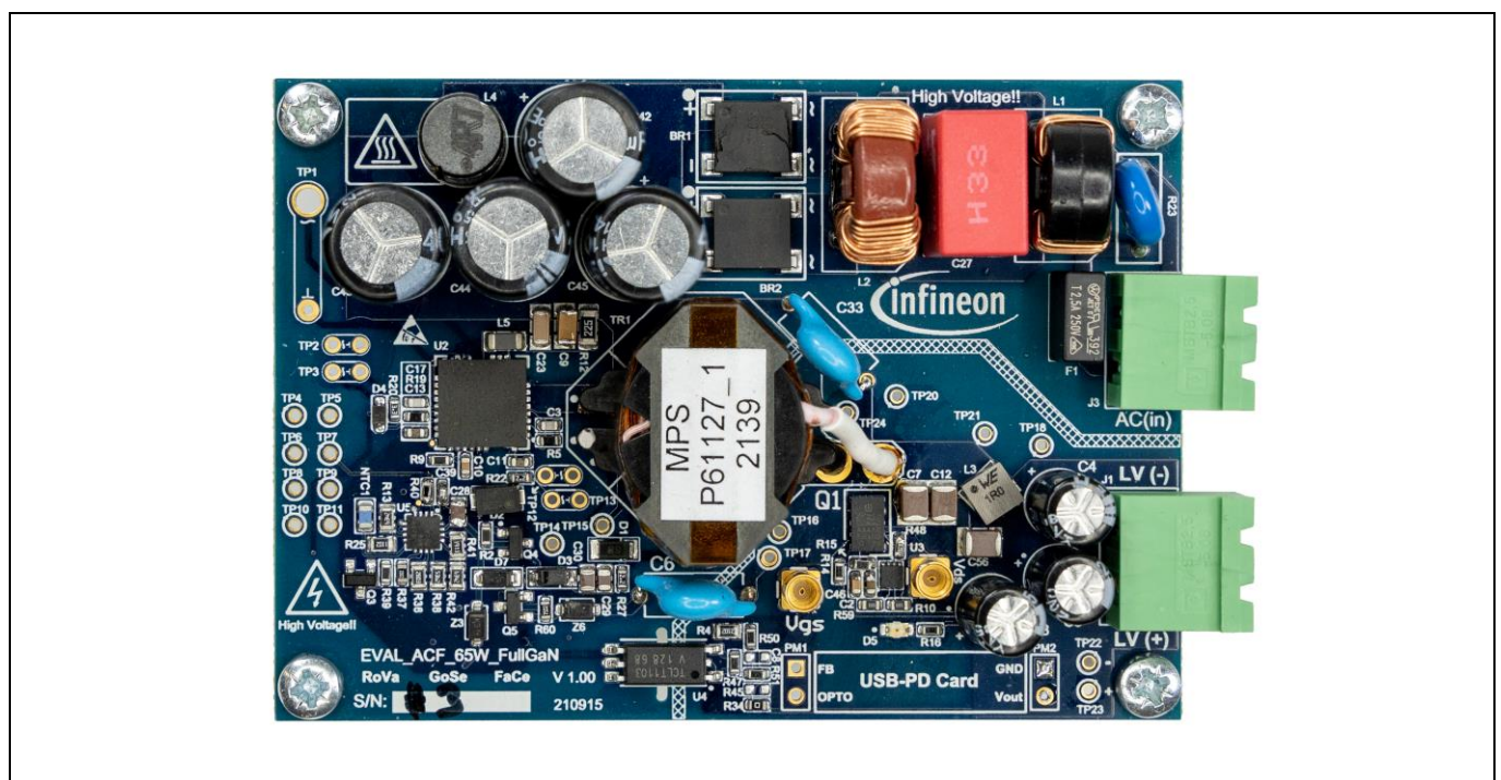
Figure 1 Full GaN 65 W ACF evaluation board featuring ICQ800NLS CoolGaN™ SG HEMT
