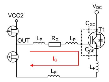
Figure 5 Gate loop with parasitics
