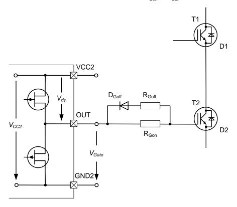
Figure 8 Basic gate circuit
