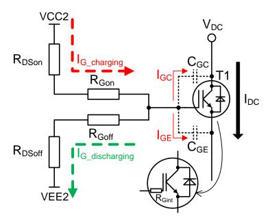
Figure 2 Gate charging/discharging diagram
