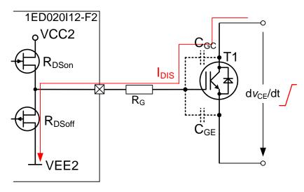
Figure 6 Parasitic tun-on
