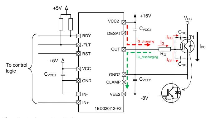
Figure 1 Basic gate driver circuit
