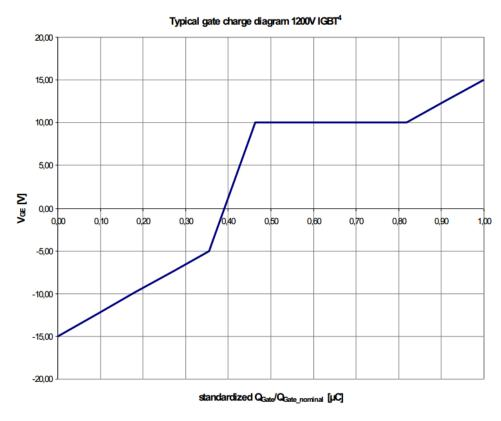
Figure 3 Gate charge diagram
