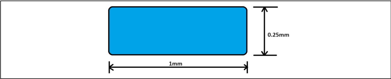
Figure 14 QFN pad size
