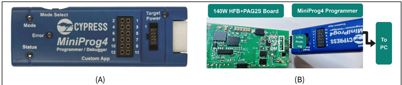
Figure 4 (A) PSoC™ MiniProg4 (CY8CKIT-005) Programmer Kit and (B) Programmer Kit connection with provision jumper
