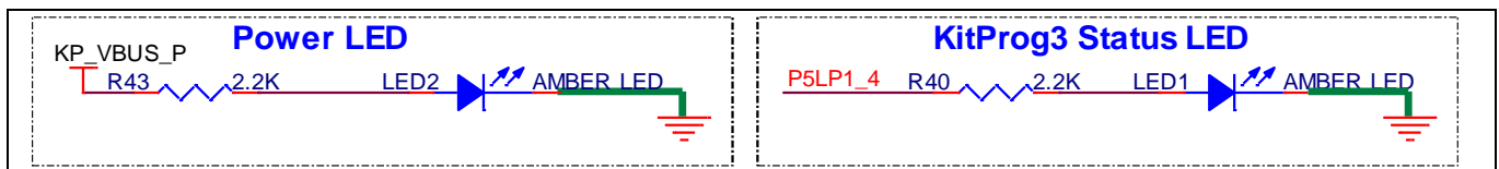
Figure 12 KitProg3 power and status LED
