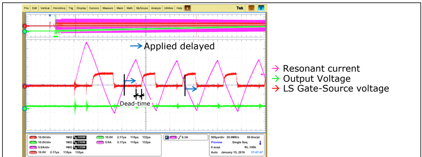
Figure 27 LS-HS driving signal change is applied with a delay after the resonant current crosses zero to guarantee current polarity change and avoid hard-commutation.
