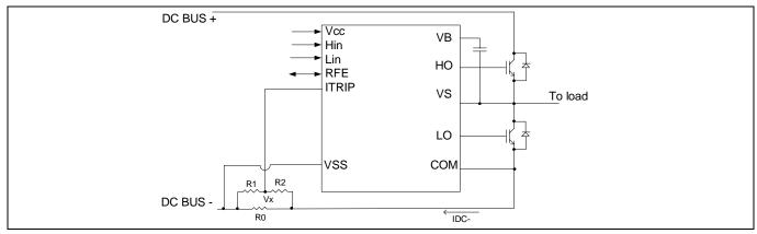
Figure 2 Typical connection of the 6ED2230S12T gate driver IC
