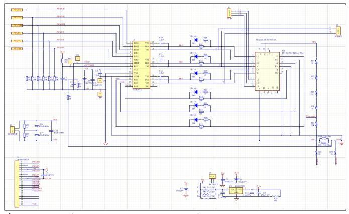
Figure 5 Schematic of the EVAL-M1-6ED2230-B1 evaluation board
