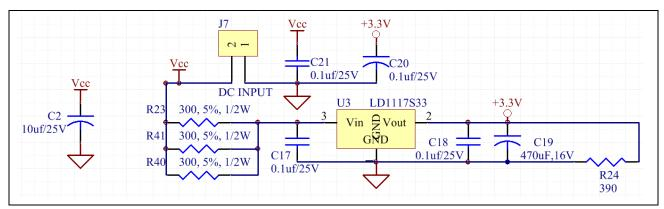
Figure 7 Power supply section of the EVAL-M1-6ED2230-B1 evaluation board
