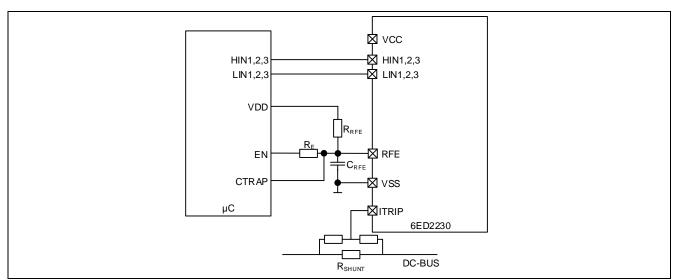
Figure 8 Overcurrent protection circuit on the EVAL-M1-6ED2230-B1 evaluation board
