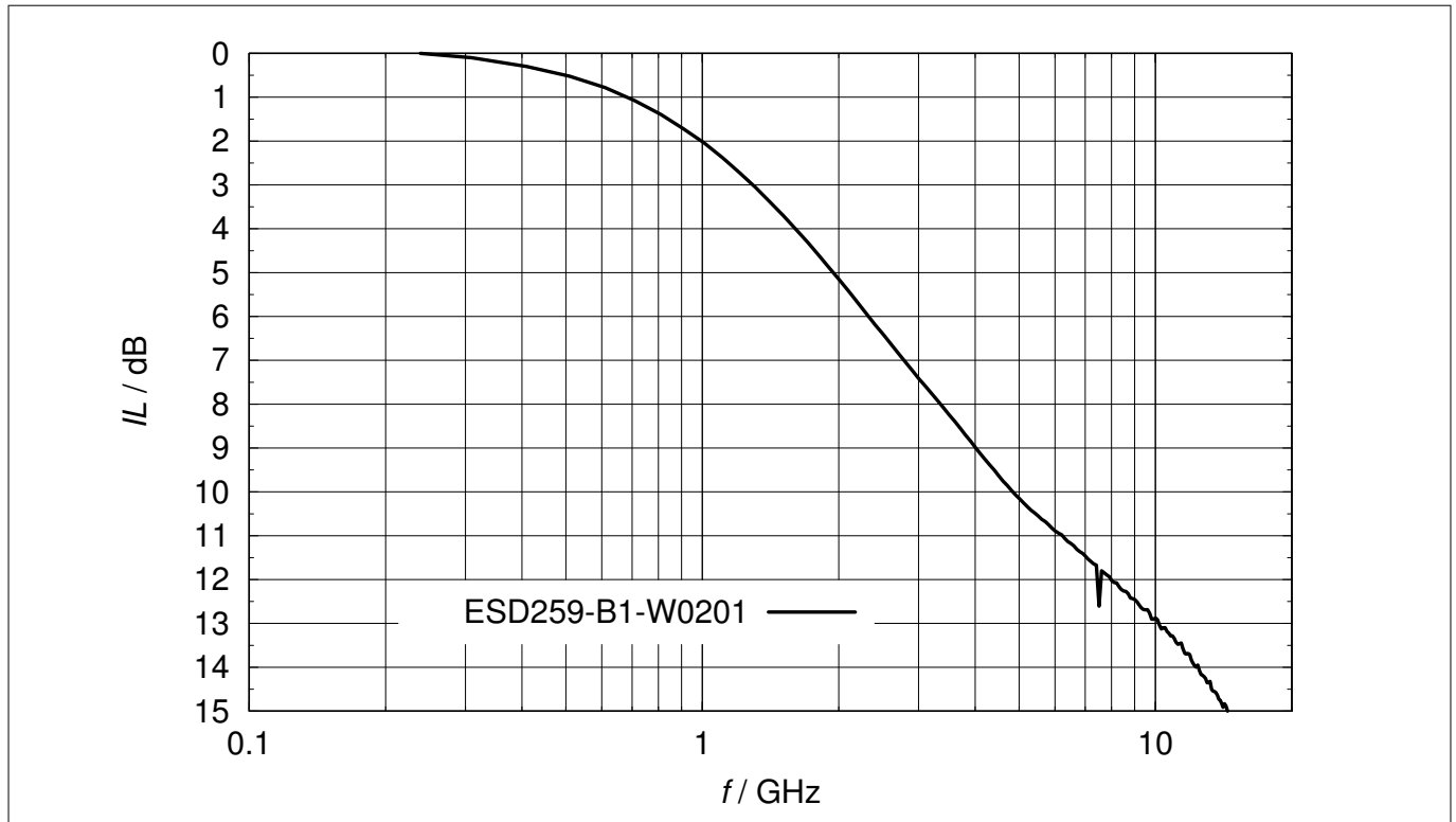
Figure 11 Insertion loss: IL = f(f)
