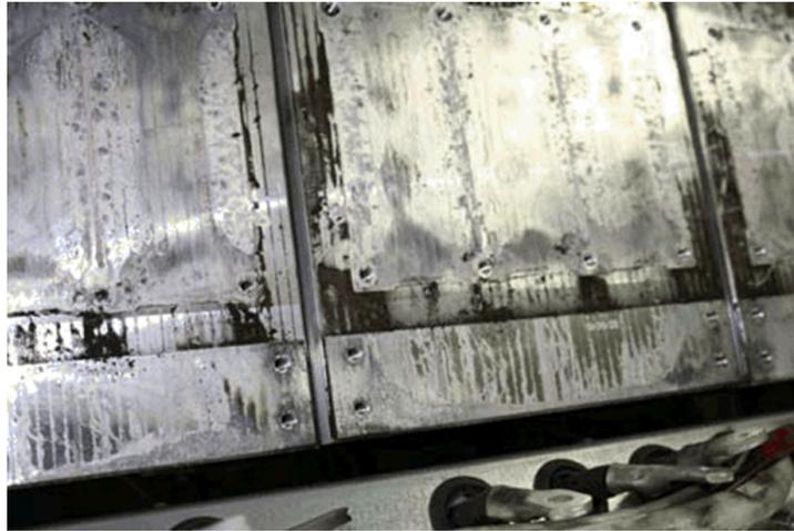
Figure 8: Heat sink of a failed inverter with no thermal grease remaining below the power module's hot spot
