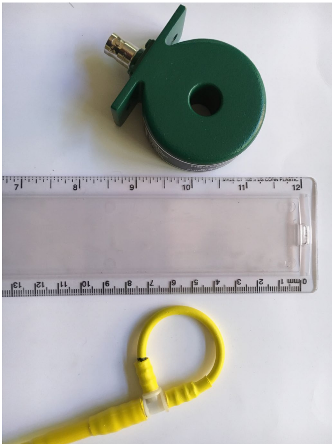
Figure 10: An example of a Pearson (left) and Rogowski coil (right) current sensor
