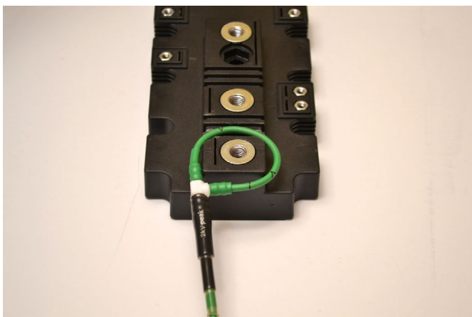
Figure 8: Rogowski coil fitted around the terminal of a PrimePACK™ 2 module
