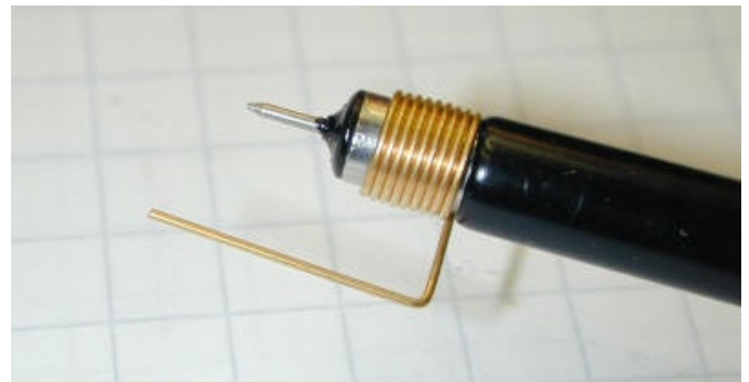
Figure 4: Voltage probe tip to reduce inductance in measurement loop
