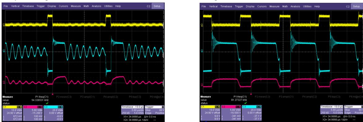
**Figure 3 Voltage at the gate (CH1, upper curve), auxiliary winding (CH3, middle curve) and ZC pin (CH2, lower curve) at light load (left) and heavy load (right)**
