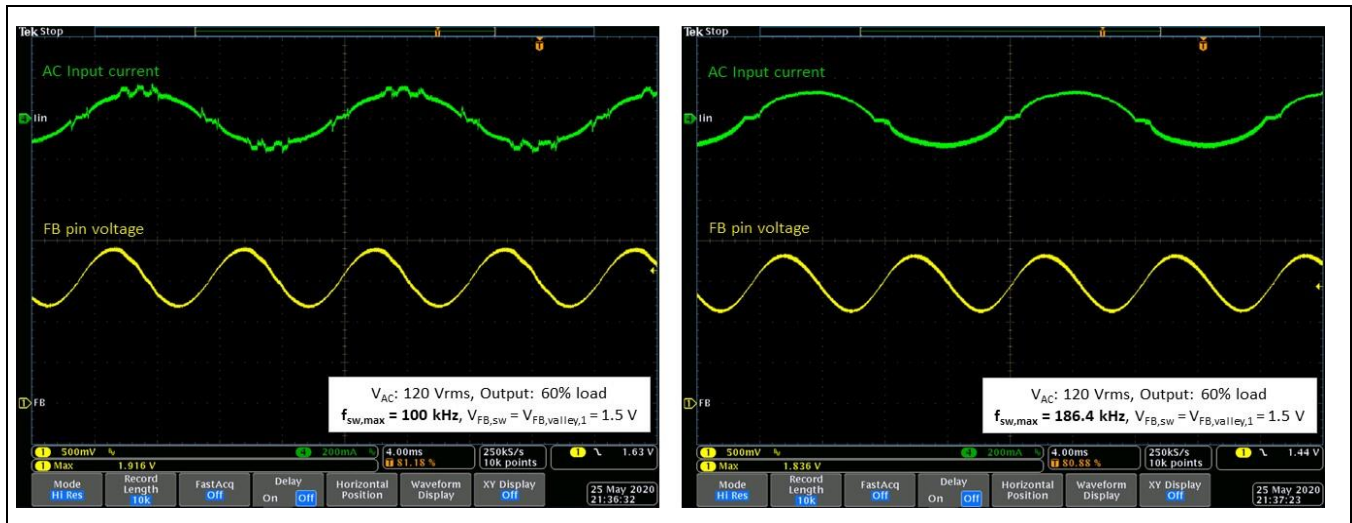
Figure 29 Input current glitches (distortion), when f_{sw,max} is too low
