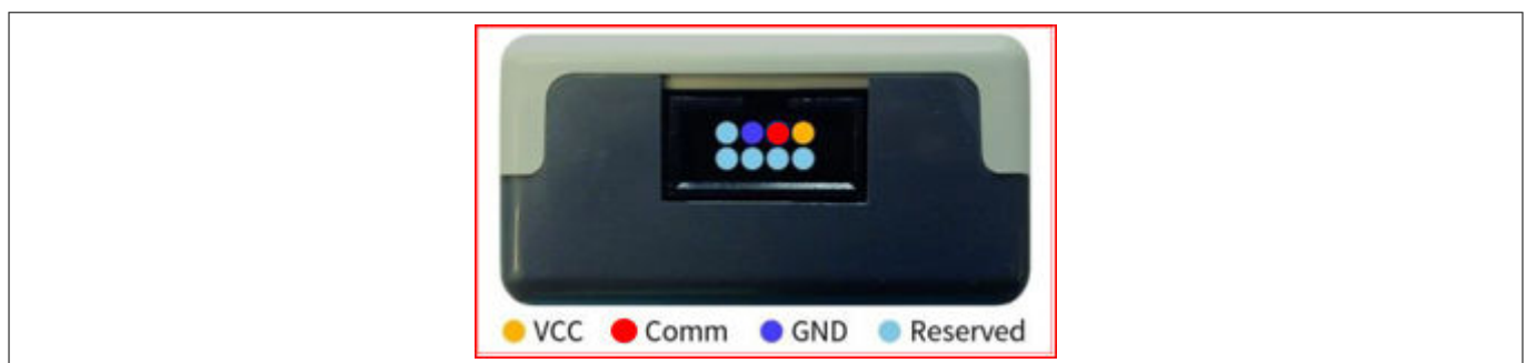
Figure 19 8-Pin connector to the target control IC
