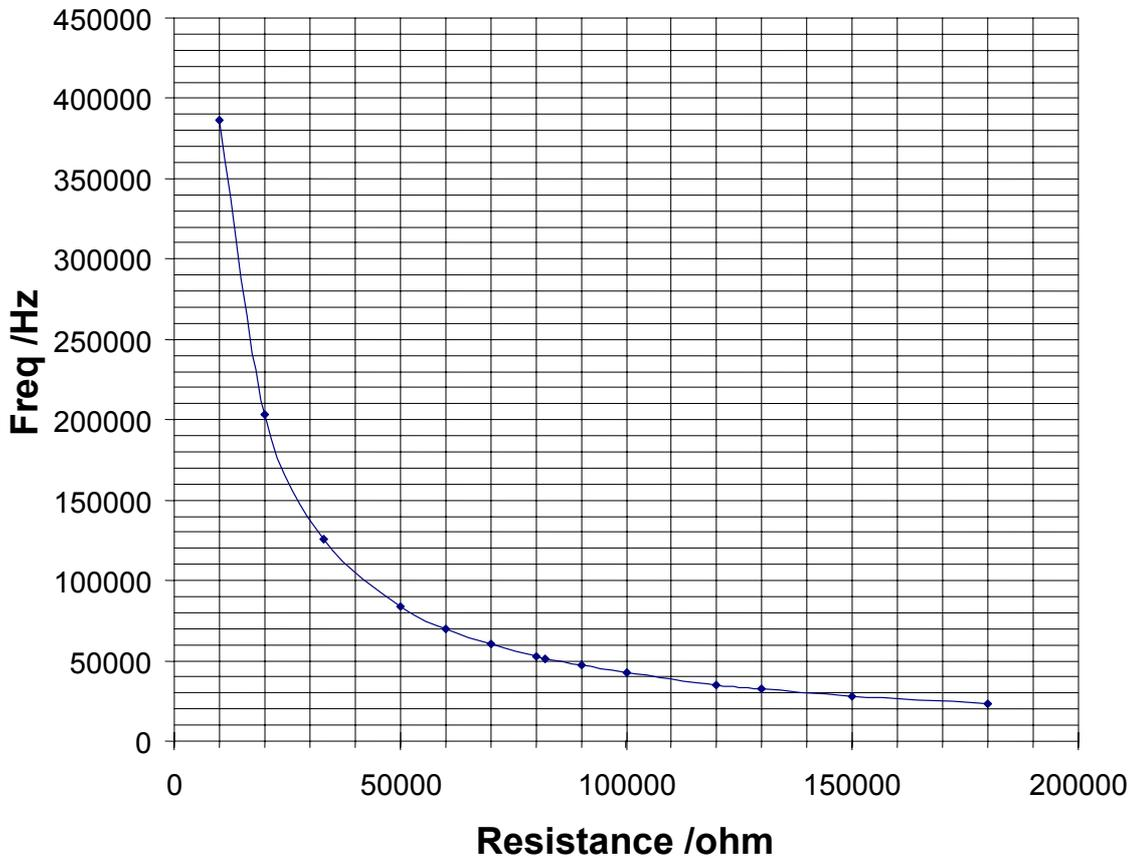
Figure 6 Resistor-frequency characteristic
