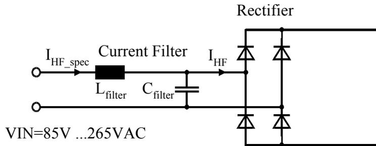
Figure 5 AC line current filter
