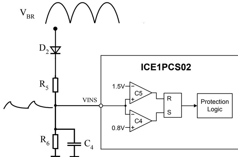
**Figure 7 Block diagram of voltage loop**
