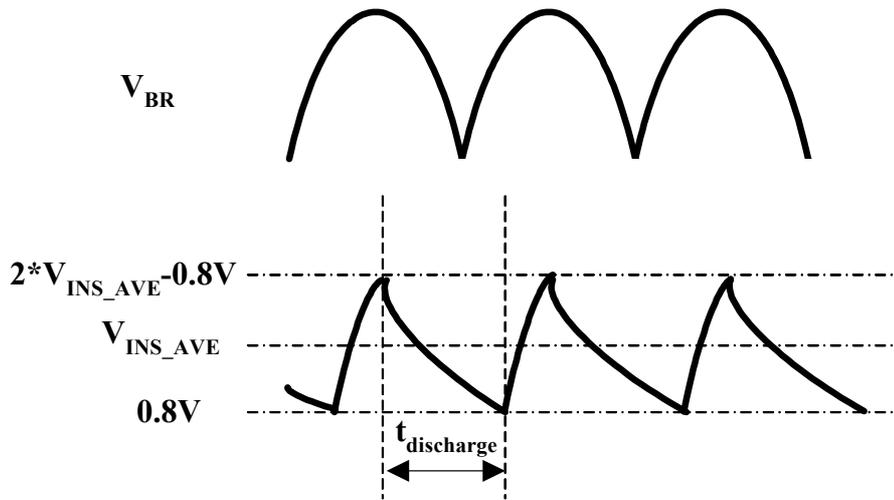
**Figure 8 Timing diagram of VINS Pin when IC enters brown-out shutdown**
