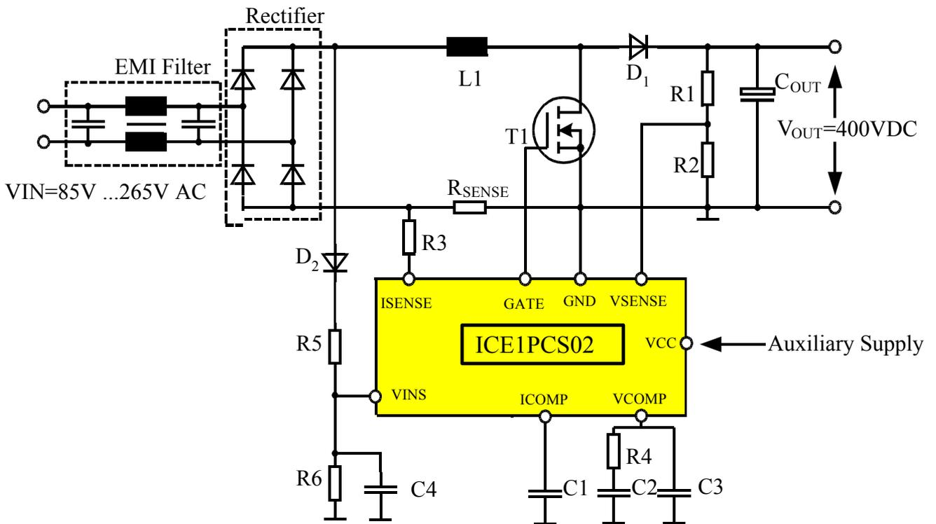
Figure 3 Typical application circuit of ICE1PCS02
