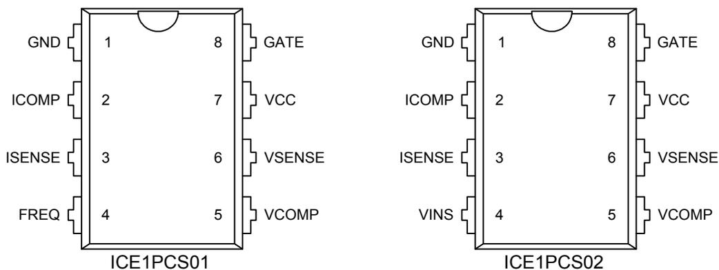
**Figure 1 Pin Layout of ICE1PCS01 and ICE1PCS02**
