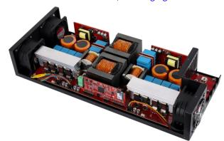
Purchase the reference design for 11 kW SiC bi-directional DC/DC converter board for EV Charging and ESS applications: <u>REF-DAB11KIZSICSYS</u>
