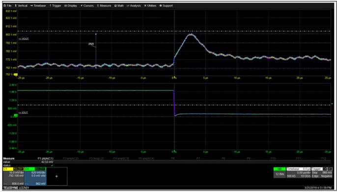
Figure 16 Transient load release from 130 A to 10 A in 200 ns
