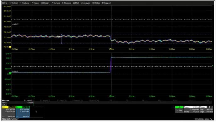
Figure 15 Transient load step from 10 A to 130 A in 200 ns
