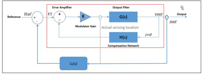
Figure 10 High-level-control-block diagram of a voltage-mode buck converter with LL
