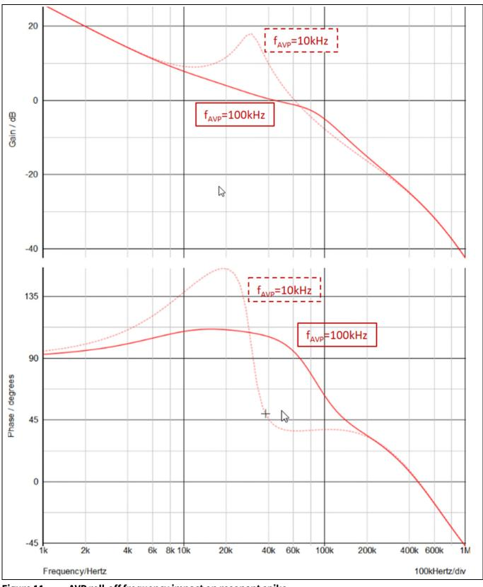
Figure 11 AVP roll-off frequency impact on resonant spike
