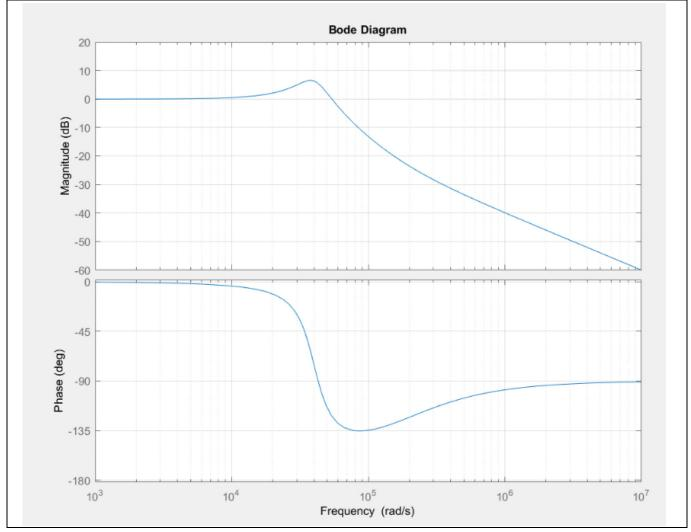
Figure 9 Bode plot of the output filter of the voltage regulator
