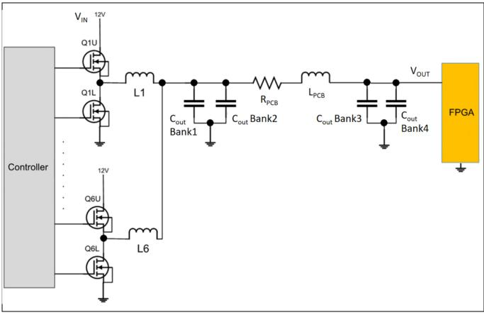
Figure 1 Overview of the Power Delivery Network (PDN) of a six-phase buck converter
