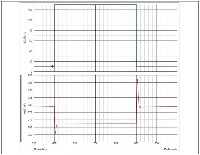
Figure 12 Transient response with 97.5  $\mu\Omega$  of LL
