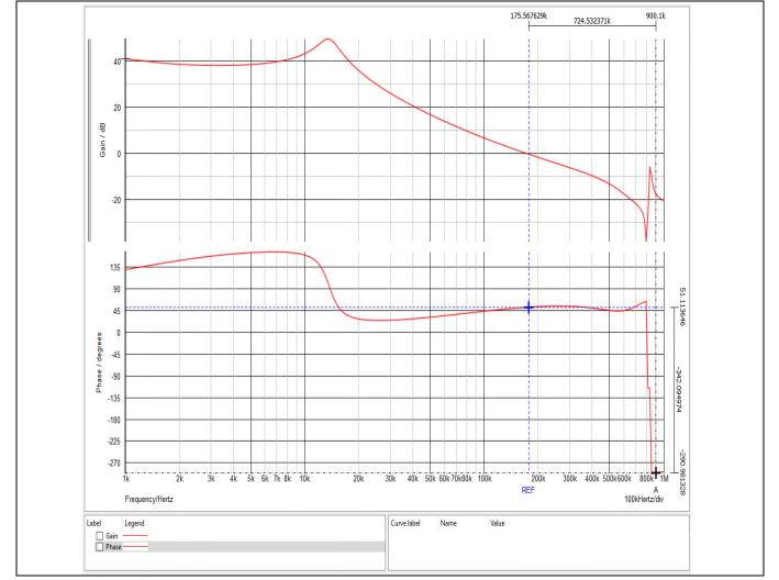
Figure 5 Simulated Bode plot of the six-phase controller without LL enabled
