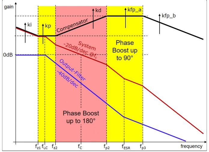
Figure 7 Linearized frequency response of a voltage-mode-controlled buck converter at no LL
