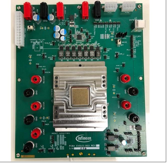
Figure 3 Picture of the PXE1610C demo board used for hardware testing and verification
