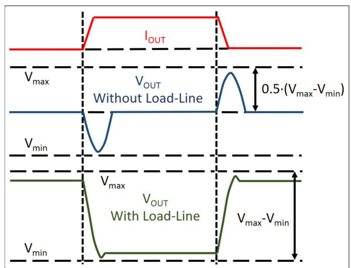
Figure 2 V<sub>out</sub> behavior during a transient event with and without LL
