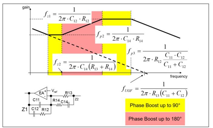
Figure 6 PID compensation network with Type III analog error amplifier
