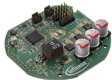
Figure: Reference design for 150W coolant pump
