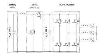
Figure 4: A typical converter topology for utility-scale
