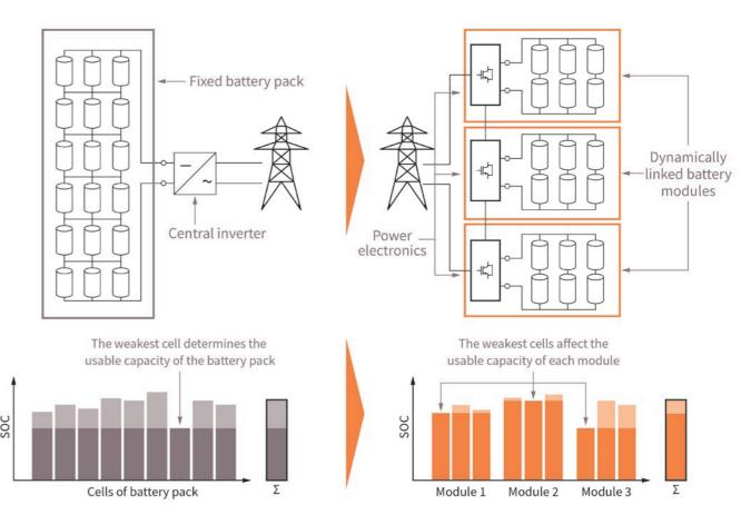
Figure 5: Battery-charge flexibility in cascaded modular multilevel ESS
