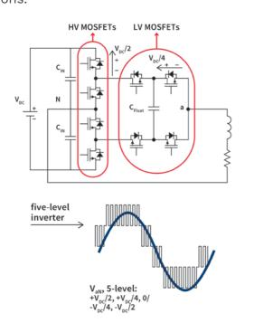
Figure 3: 5-level flying capacitor active neutral point clamp inverter basic schematic
