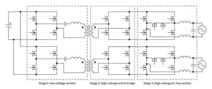
Figure 2: A possible converter topology for residential ESS
