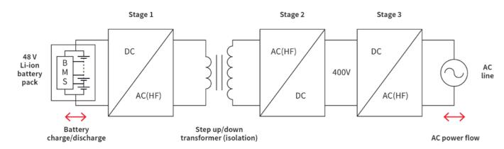
Figure 1: Basic block diagram for a residential energy storage system
