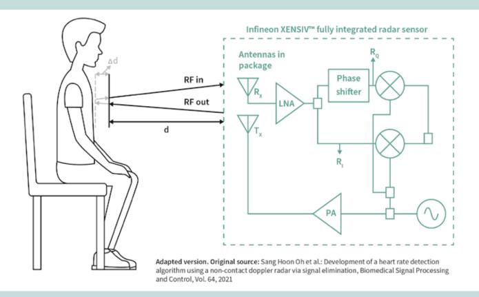
Figure 2: Operating principle of radar technology for vital sensing
