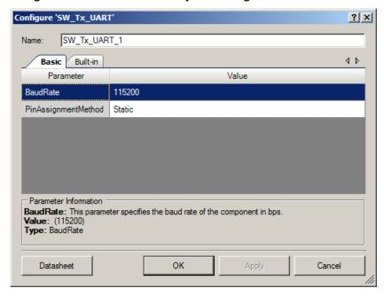
The SW\_Tx\_UART provides the following parameters.
