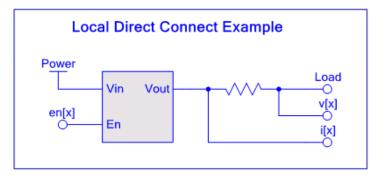
The diagram below shows the connection methodology for a power converter that has an output voltage > Vdda. An external current sense amplifier (CSA) is required to convert the differential voltage drop across the sense resistor to a single-ended voltage that connects directly to this component. The voltage sense point is scaled down to a voltage level that can directly connect to this component.
