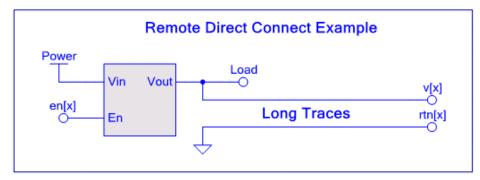
The diagram below shows the connection methodology for a remote power converter that has an output voltage > Vdda where the remote voltage sense point is scaled using resistors and is routed back to this component along with the remote ground reference point.
