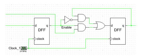
If access to a clock is needed, for example to generate a clock to send to a pin, then a 2x clock should be used to clock a toggle flip-flop. The output of that flip-flop can then be used with the associated timing analysis available.
