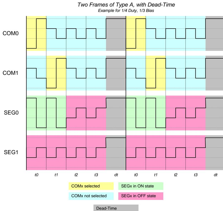
This illustration shows the principle for 1/3 bias and 1/4 duty implementation, but the general approach of reducing contrast by reducing the percentage of time the glass is driven can be generalized and applied to any drive method.
