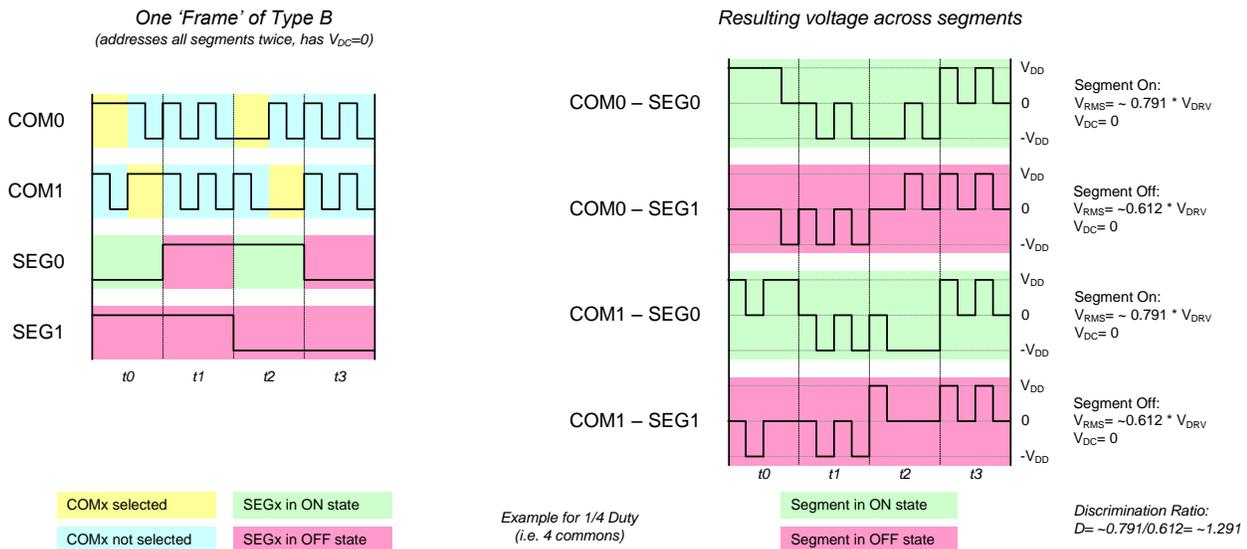
As illustrated, instead of generating bias voltages between the rails, this approach takes advantage of the characteristic of the LCD displays; the degree of on-ness and off-ness of LCD
