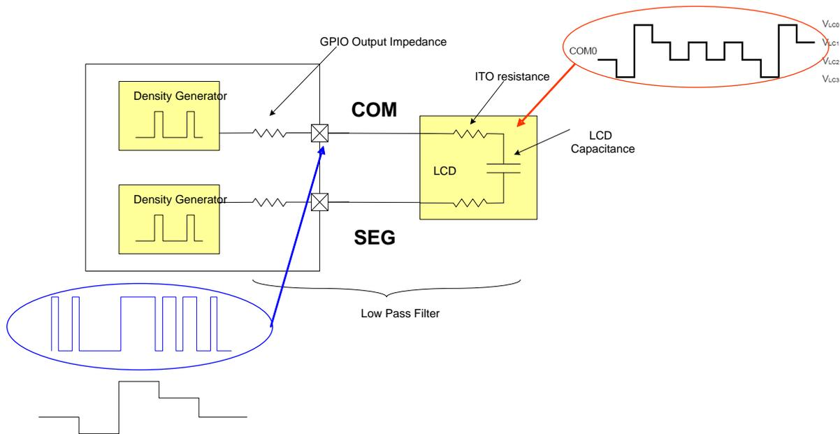
In order to drive a low capacitance display with acceptable ripple and rise/fall time using a 32 kHz PWM an additional external series resistance of 100 k - 1 M ohm is required. External Resistors are not required for PWM frequencies of greater than ~1 MHz. The exact frequency depends on the capacitance of the display, the internal ITO resistance of the ITO routing traces, and the drive impedance of the I/O pins.
