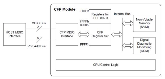
The MDIO Host uses this interface to control and monitor the startup, shutdown and normal operation of the CFP modules it manages. At the same bus, multiple slaves can be connected to the same host with different bus addresses. The address of the module can be configured through the Port Address bus.
