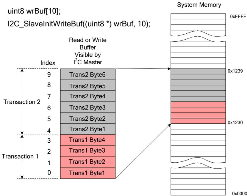
Both the read and write buffers have four status bits to signal transfer complete, transfer in progress, and buffer overflow. Starting a transfer sets the busy flag. When the transfer is complete, the transfer complete flag is set and the busy flag is cleared. If a second transfer is started, both the busy and transfer complete flags can be set at the same time. The following table shows read and write status flags.
