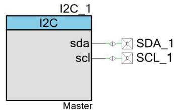
**UDB I<sup>2</sup>C Slave with Clock and Pins**
