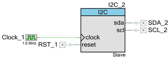
**UDB I<sup>2</sup>C Master with Clock and Pins**
