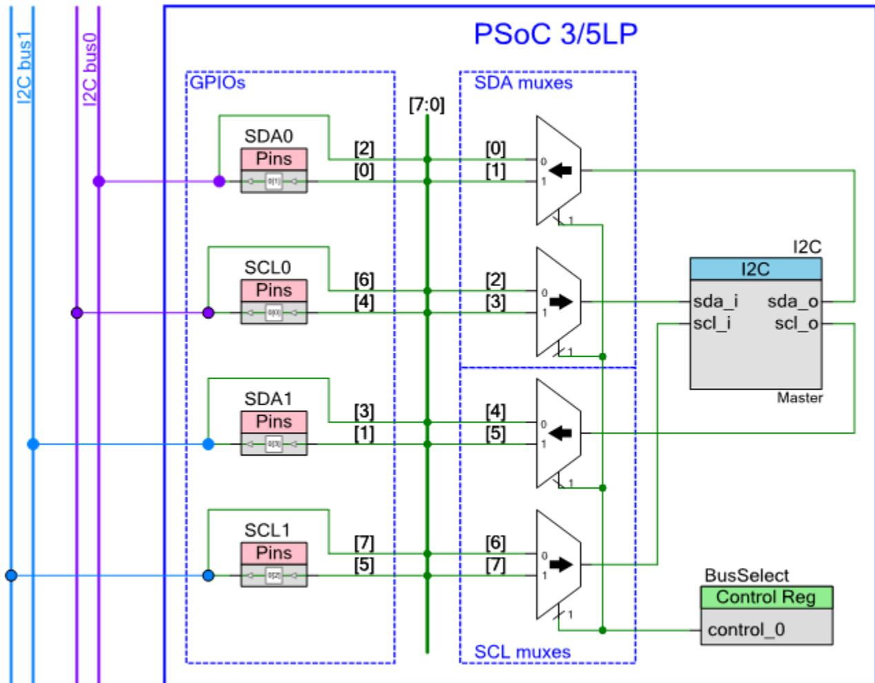
Figure 8 shows the PSoC Creator schematic which implements sharing of single I<sup>2</sup>C bus with two I<sup>2</sup>C components inside PSoC. It can be extended to support multiple components to share the same bus. The I2C1 and I2C2 components sense the same inputs and their outputs are ANDed together to drive the bus.
