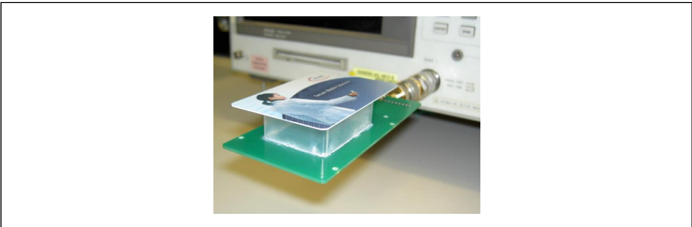
Figure 17 Setup for unloaded resonance frequency measurement
