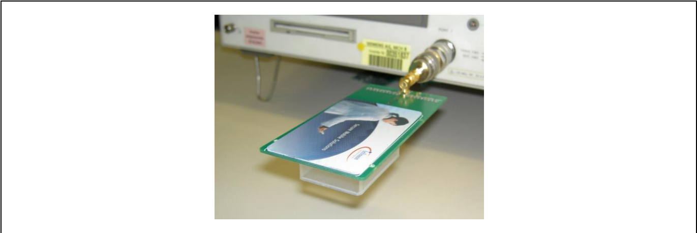
Figure 15 Setup for threshold resonance frequency measurement
