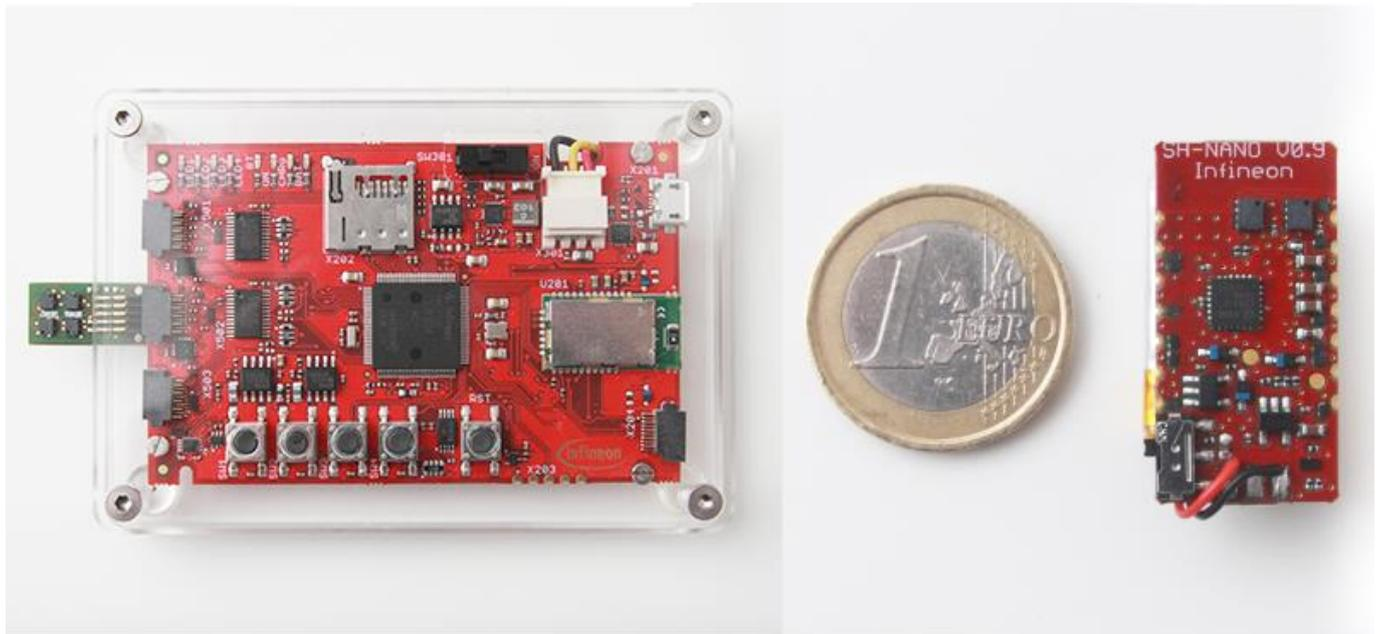
**Figure 4. Sensor Hub evaluation environments support design-in of DPS310 pressure sensors**
