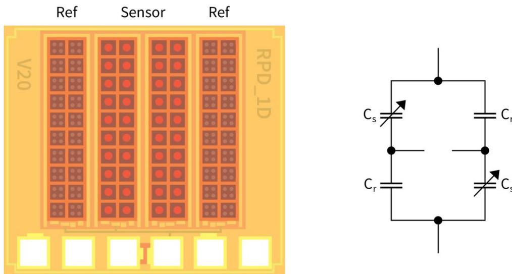
**Figure 1. Capacitive pressure sensing cell structure and bridge configuration**
