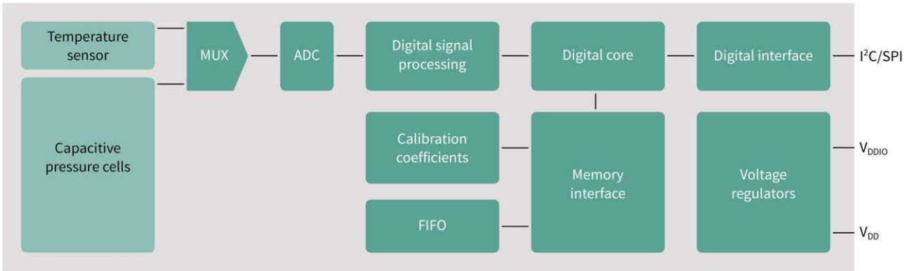
**Figure 2. DPS310 functional block diagram**
