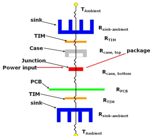
Fig. 3 Different options for usage of a heatsink.
