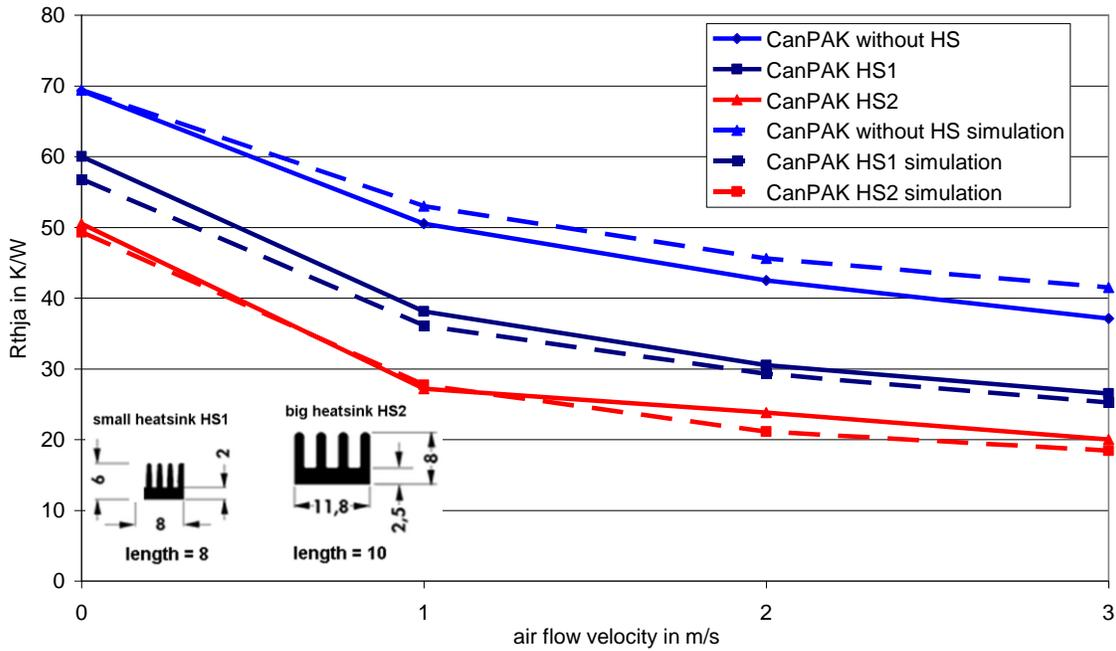
Fig. 8 Measurement and simulation results  $R_{thJA}$  – CanPAK™ with and without heatsink
