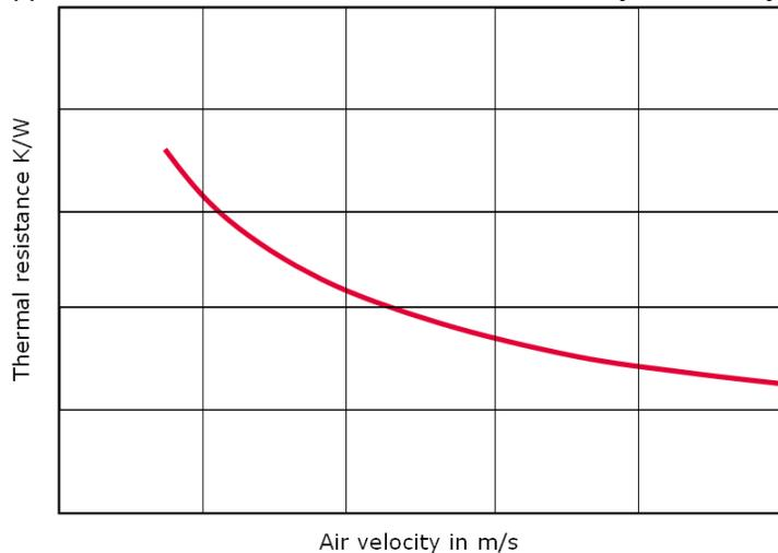
Fig. 5 Typical performance graph of a heatsink
