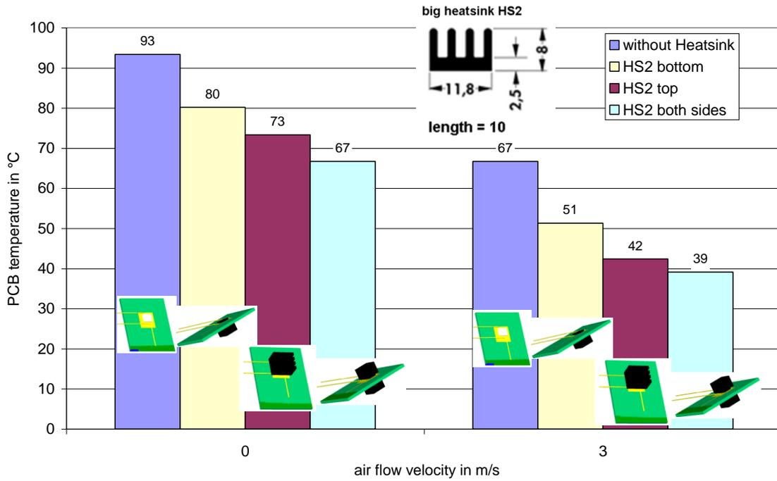
Fig. 11 Simulation results for PCB temperature (Power dissipation 1 W, ambient temperature 25°C)
