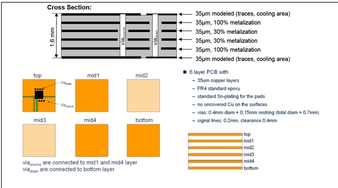
Fig. 14 PCB board used for thermal measurement and simulation
