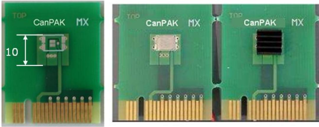
Fig. 7 Measurement boards (dimensions in mm)
