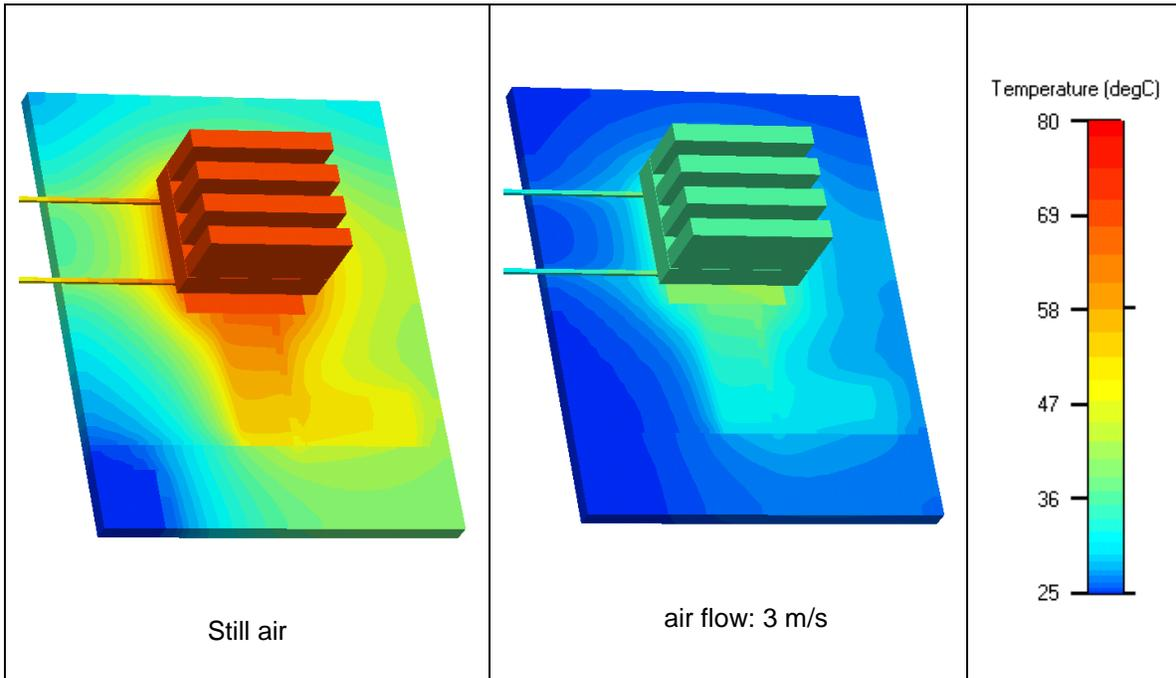
Fig. 13 Simulation results for PCB temperature (Power dissipation 1 W, ambient temperature 25°C, heatsink HS2)
