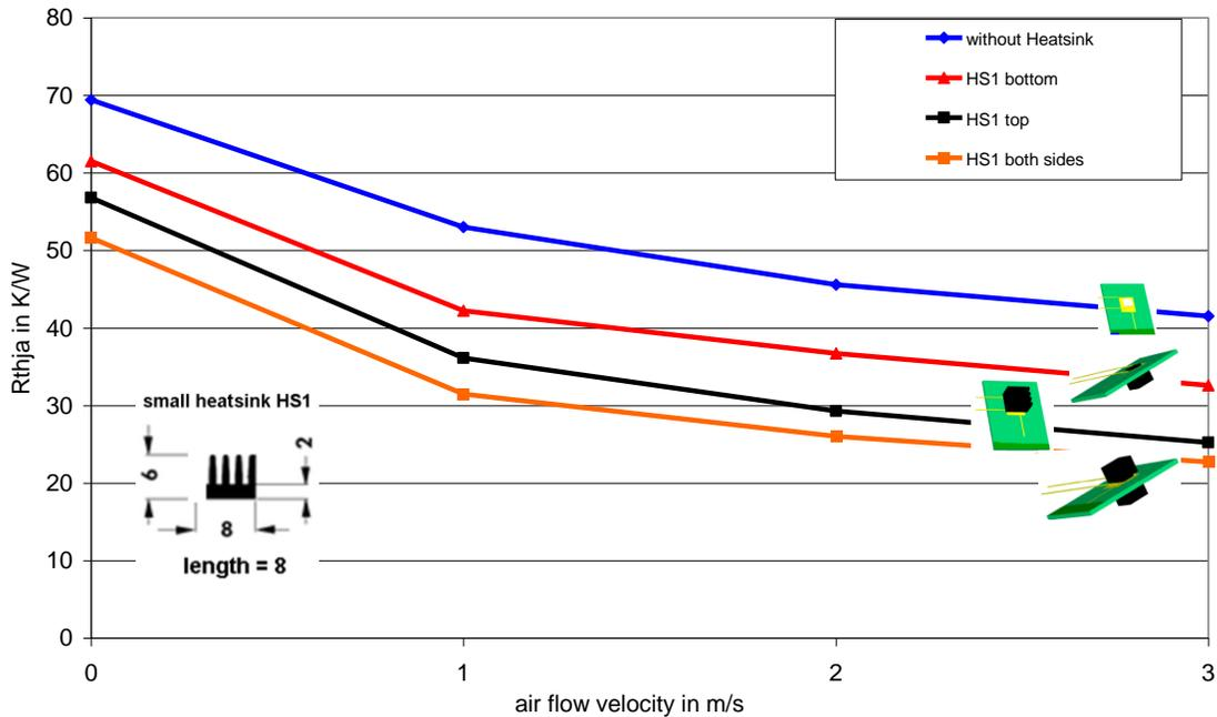
Fig. 10 Simulation results  $R_{thJA}$  – CanPAK™ with and without heatsink and different arrangements of the heatsink
