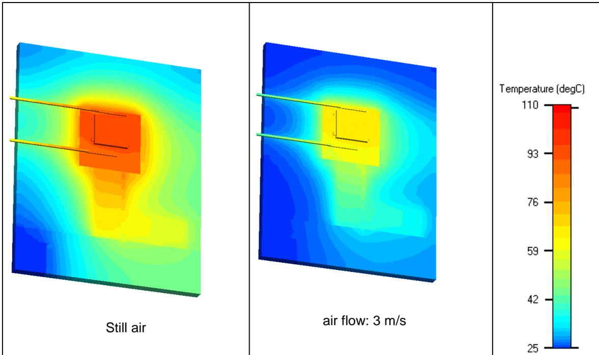
Fig. 12 Simulation results for PCB temperature (Power dissipation 1 W, ambient temperature 25°C)
