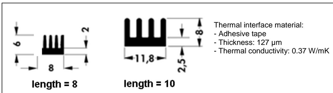
Fig. 6 Heatsinks used for measurement and simulation (left: heatsink HS1, right: Heatsink HS2, dimensions in mm)
