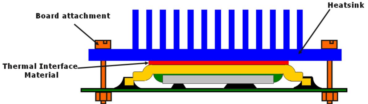
Fig. 4 Using a heatsink (heatsink, thermal interface material (TIM) and board attachment)
