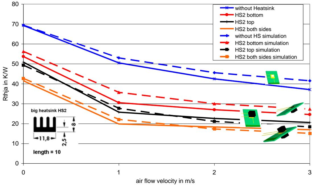
Fig. 9 Measurement and simulation results  $R_{thJA}$  – CanPAK™ with and without heatsink and different arrangements of the heatsink
