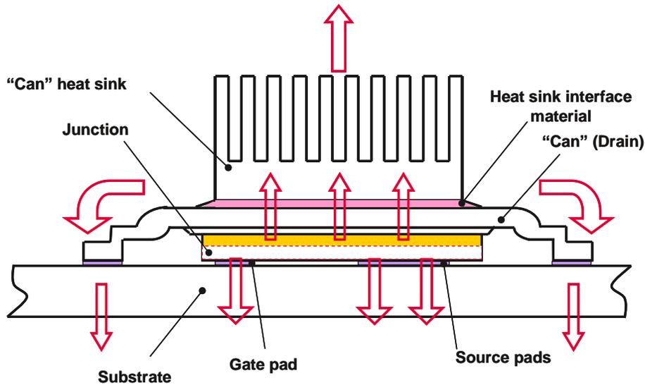
Fig. 2 CanPAK showing heatflow directions (red arrows)
