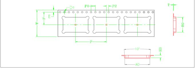
Figure 20 CYBLE-3x307x-02 tape dimensions
