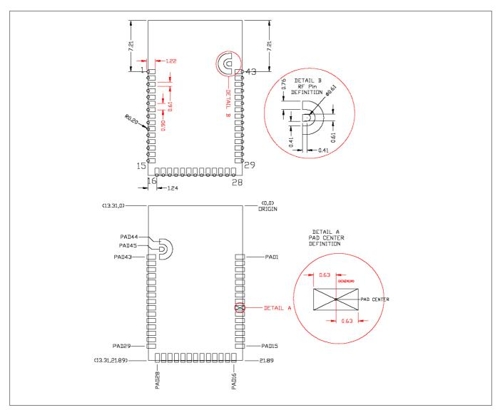
Figure 7 Solder pad reference location
