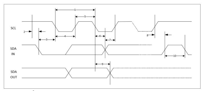
Figure 16 I<sup>2</sup>C Interface timing diagram
