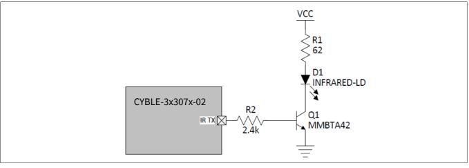
Figure 11 Infrared TX
