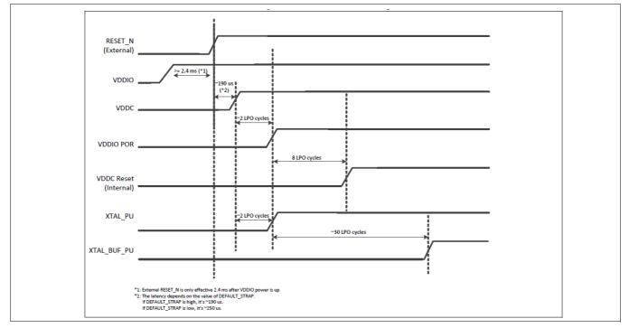
Figure 10 Power-on reset timing
