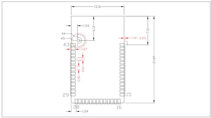
Figure 5 CYBLE-3x307x-02 host layout (dimensioned)
