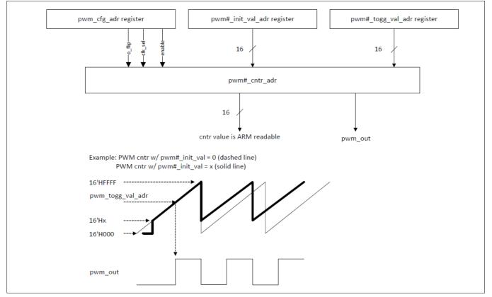
Figure 12 PWM block diagram
