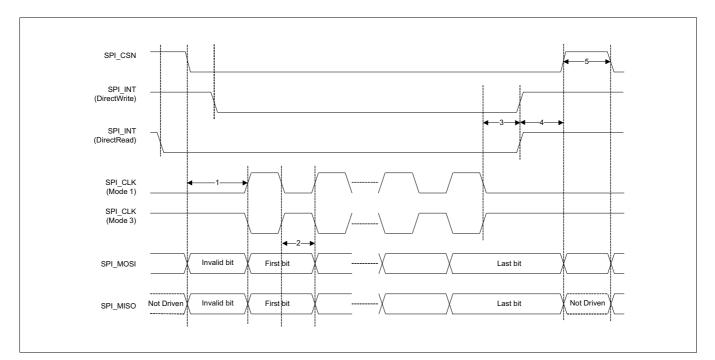
Figure 15 SPI timing – mode 1 and 3
