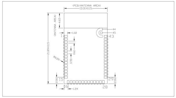
Figure 3 Solder pad dimensions (seen from bottom)
