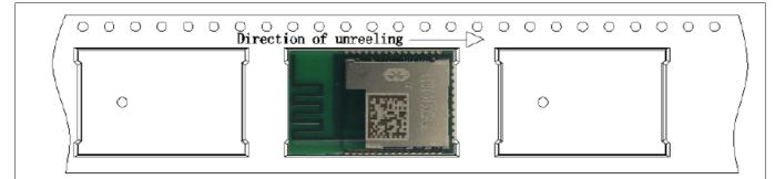
Figure 21 Component orientation in tape and unreeling direction
