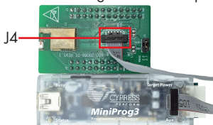
Fig 3: Programming/Debugging with MiniProg3
