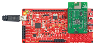
Fig 4: Programming and debugging with CY8CKIT-042-BLE BLE Pioneer Kit Baseboard
