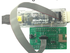
Fig 3: Programming/Debugging with MiniProg3
