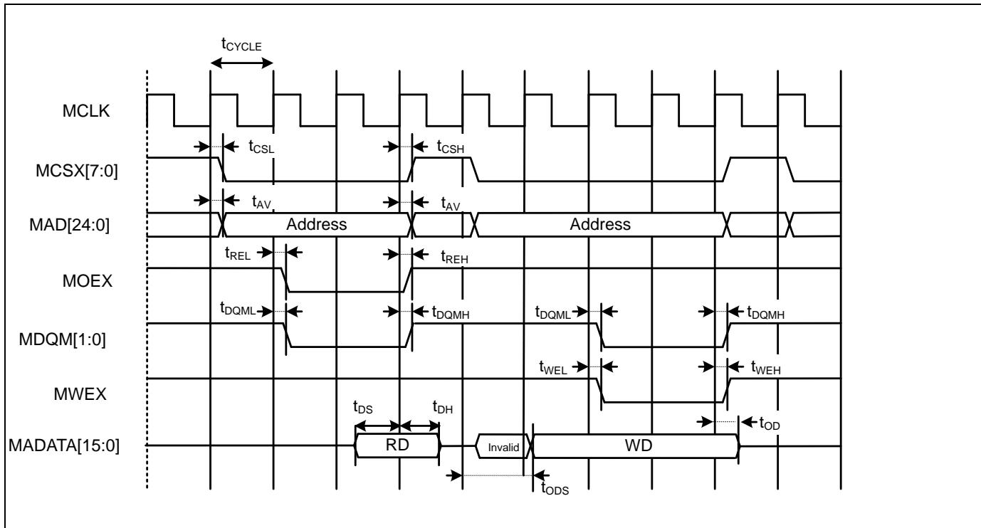
**Multiplexed Bus Access Asynchronous SRAM Mode**
