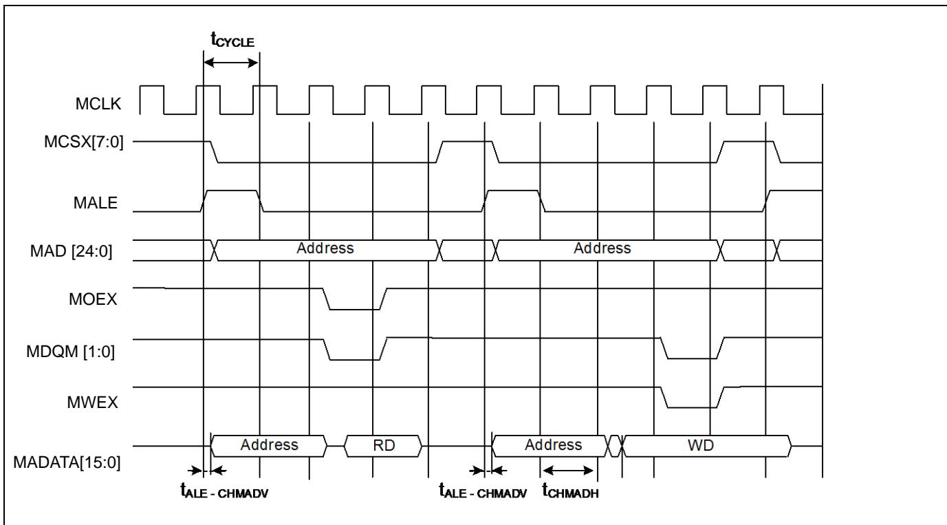
**Multiplexed Bus Access Synchronous SRAM Mode**
