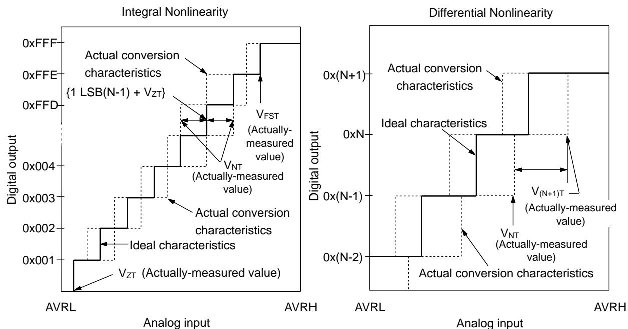
$$\text{Integral Nonlinearity of digital output } N = \frac{V_{NT} - \{1\text{LSB} \times (N - 1) + V_{ZT}\}}{1\text{LSB}} \text{ [LSB]}$$
