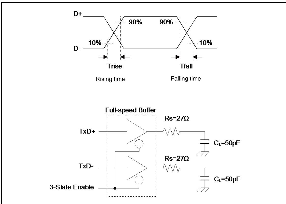
\*6: USB Full-speed connection is performed via twist pair cable shield with  $90\Omega \pm 15\%$  characteristic impedance (Differential Mode). USB standard defines that output impedance of USB driver must be in range from  $28\Omega$  to  $44\Omega$ . So, discrete series resistor ( $Rs$ ) addition is defined in order to satisfy the above definition and keep balance.
