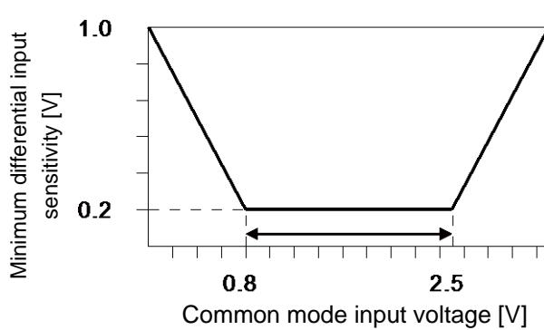
\*3: The output drive capability of the driver is below 0.3 V at Low-State ( $V_{OL}$ ) (to 3.6 V and 1.5 k $\Omega$  load), and 2.8 V or above (to ground and 15 k $\Omega$  load) at High-State ( $V_{OH}$ ).
