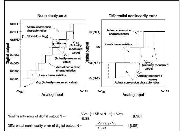
$1LSB = \frac{V_{FST} - V_{OT}}{1022}$
