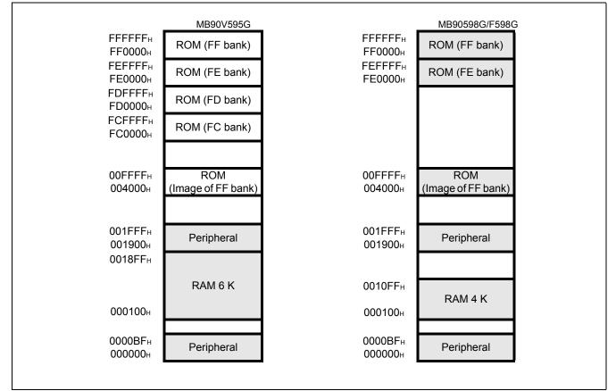
Note: The ROM data of bank FF is reflected in the upper address of bank 00, realizing effective use of the C compiler small model. The lower 16-bit of bank FF and the lower 16-bit of bank 00 are assigned to the same address, enabling reference of the table on the ROM without stating "far".
