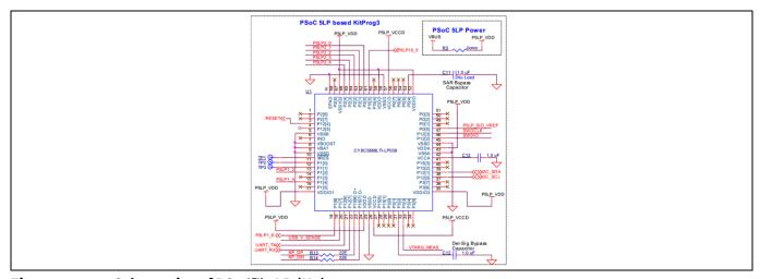
Figure 12 Schematics of PSoC™ 5LP (U1)
