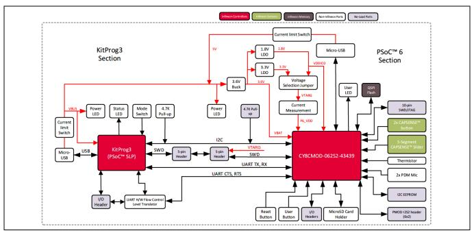
Figure 4 Block diagram of the board
