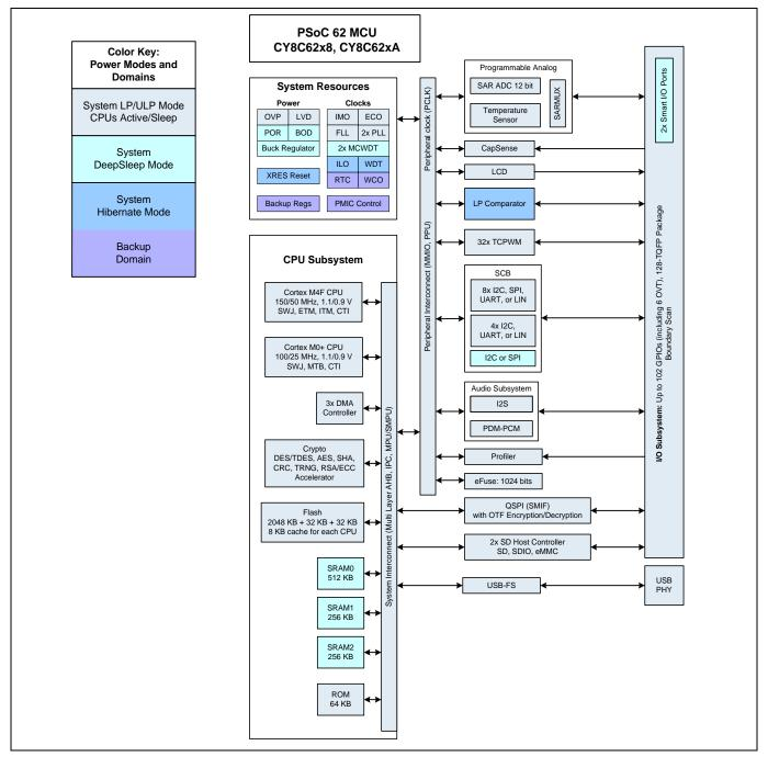
Figure 3 PSoC™ 6 MCU block diagram
