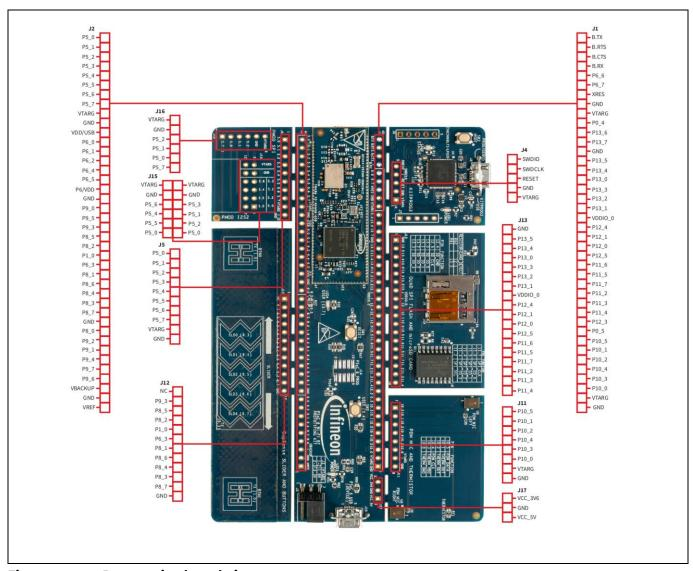
Figure 2 Prototyping board pinout
