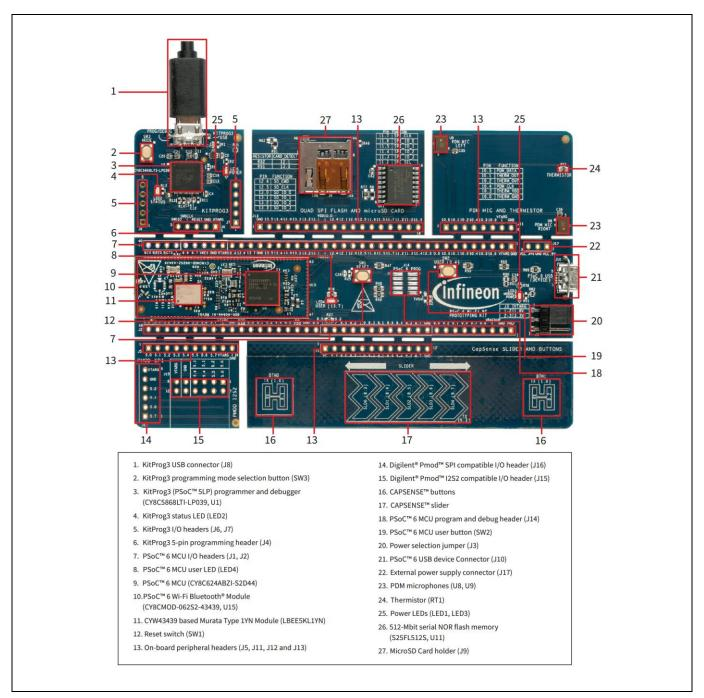
Figure 1 Board components
