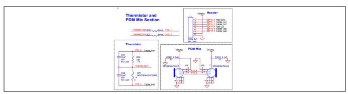
Figure 21 Schematics of PDM Mic and Thermistor
