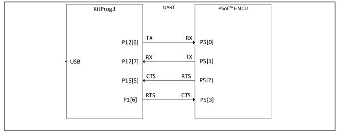
Figure 9 UART connection between KitProg3 and PSoC™ 6 MCU
