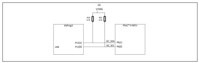
Figure 10 12C connection between KitProg3 and PSoC™ 6 MCU
