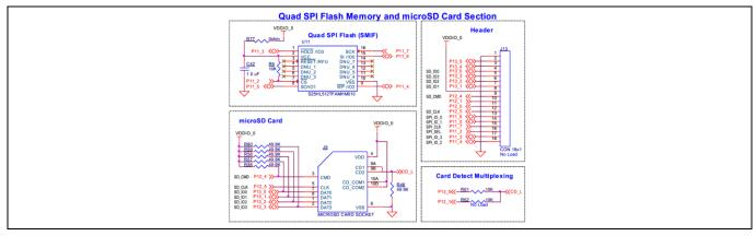
Figure 20 Schematics of Quad SPI Flash and microSD card holder
