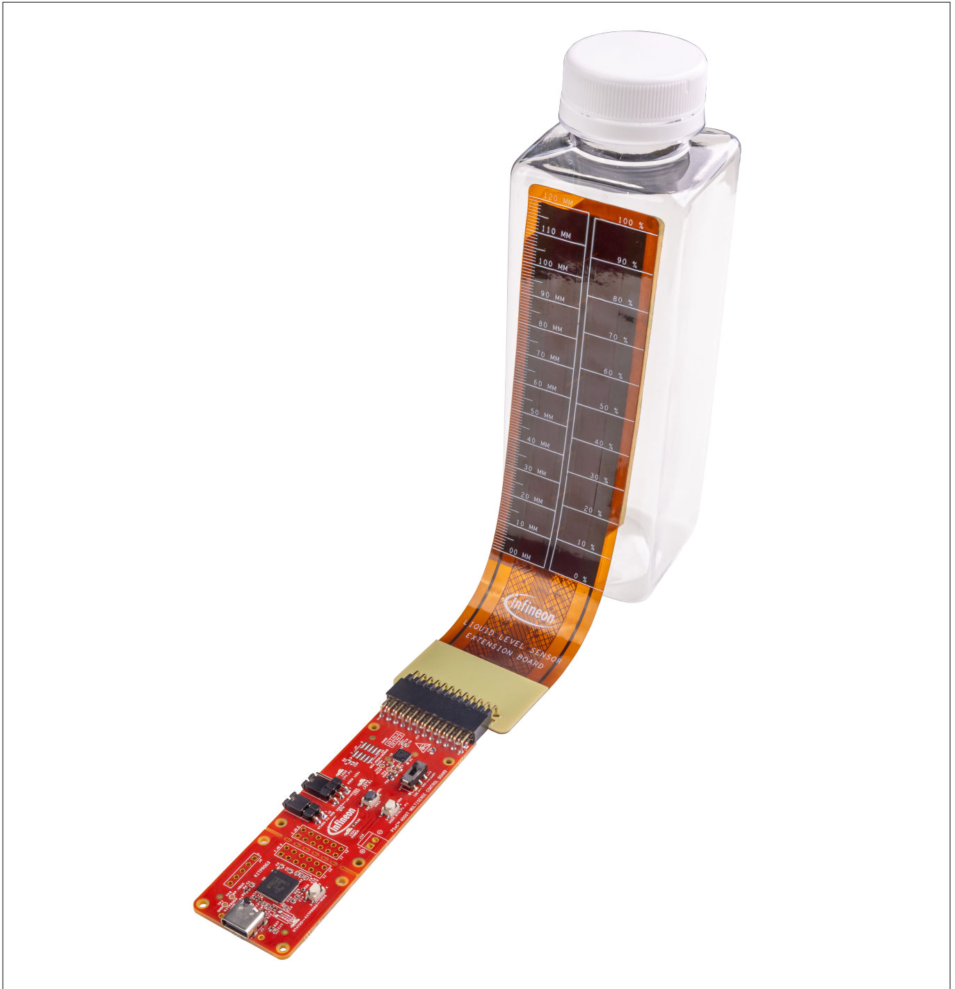
Figure 55 Liquid level sensing setup with container
