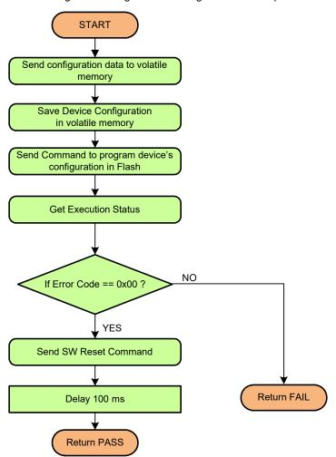
Figure 4-4. Algorithm of "Program Flash" Step
