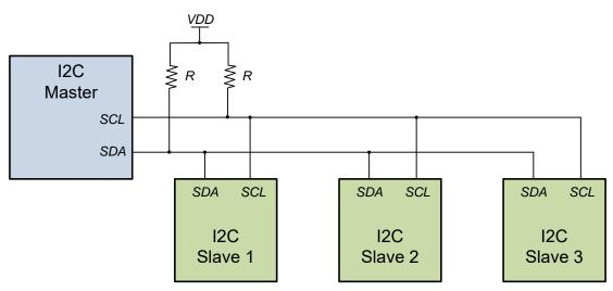
The programming flow consists of multiple Read and Write I2C transactions. These transactions are atomic transactions from the standpoint of this specification. They can be of different length in bytes, but both are embraced in the bus's START and STOP signals. Repeated START is not used.
