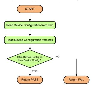
Figure 4-5. Algorithm of "Verify Flash" Step
