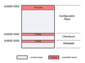
**0x0000 0000 - Configuration Data** (128 bytes), which must be programmed into the flash. These bytes configure the CY8CMBR3xxx device during boot.
