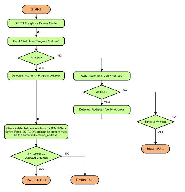
Figure 4-2. Flow Chart of Acquisition Sequence
