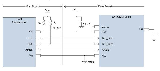
Figure 3-3. Connection Schematic of Programmer
