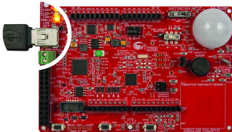
Figure 3-17. Connect USB Cable to USB Connector on the Kit
