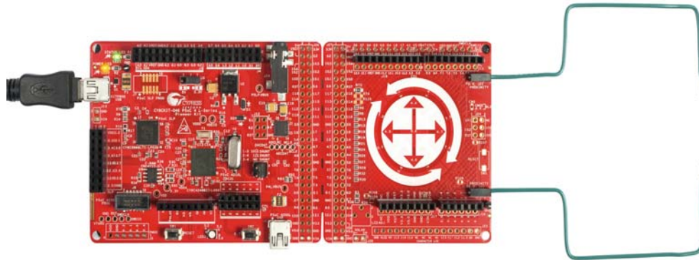
Figure 4-15. Proximity Sensor (Gestures) Connection on PSoC 4 L-Series Pioneer Kit
