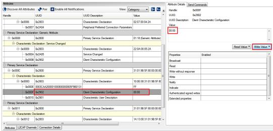
15.Locate the **RGB LED Control** characteristic (**UUID 0x0003CBB1-0000-1000-8000-00805F9B0131**). Click **Read Value** to read the existing 4-byte onboard RGB LED color information, as shown in Figure 4-20. The four bytes indicate red, green, blue, and the overall brightness, respectively.
