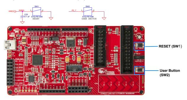
**Note**: The PSoC 4 BLE Reset pin (XRES) has an internal pull-up resistor. However, external pull-up resistor R3 and capacitor C25 are connected to PSoC 4 Reset pin on the PSoC 4 BLE Module, which is optional and required only in a noisy system.
