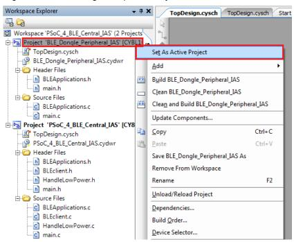
3. Program the BLE Dongle with the *BLE\_Dongle\_Peripheral\_IAS* code example described in Using Code Examples on page 37.
