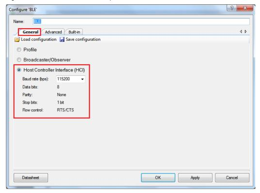
Many companies develop BLE testers for Direct Test Mode. It is also possible to create PC-based software tools that will send HCI commands over serial communication links.
