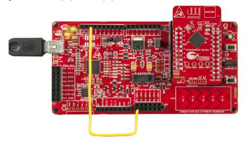
The pin assignment for this code example is in *PSoC\_4\_BLE\_Eddystone.cydwr* in the Workspace Explorer, as shown in Figure 4-58.
