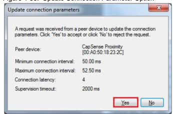
**Note:** If you select **No**, the code example will still work. However, the current consumption will be higher due to faster connection interval.
