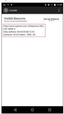
Figure 4-62. Locate Beacon Showing Details about Selected Beacon
