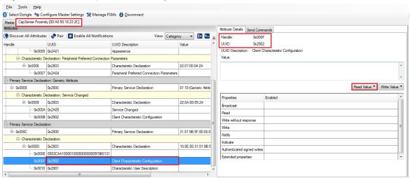
12. Modify the **Value** field to '01:00' and click **Write Value**. This enables the notifications on the Cap-Sense proximity characteristic.
