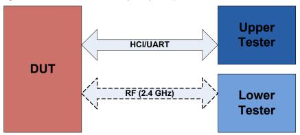
The BLE Component allows configuring the device in DTM by enabling the HCI. The appropriate responses to commands from the tester are performed by the BLE protocol stack and does not involve separate application handling. The only tasks required are to start the BLE Component and call the API to process the events.
