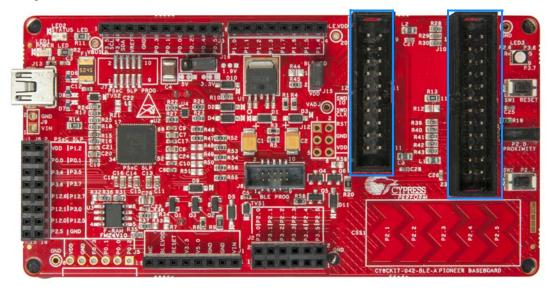
To remove the PSoC 4 BLE Module from the BLE Pioneer Kit, hold the BLE Pioneer Kit in one hand and the module in the other, as shown in Figure 3-6, and pull it out using a rocking motion.
