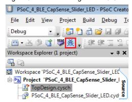
2. When PSoC Creator opens in debug mode, use the buttons on the toolbar for debugging.
