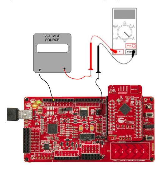
To measure the power consumption of only the module with coin cell, connect the coin cell directly to the PSoC 4 BLE Module, as shown in Figure 5-8. The BLE Pioneer Baseboard is designed with additional circuits to protect the BLE device and the F-RAM in an Arduino environment. Note that power consumption measurements on the BLE Pioneer Baseboard will also include the power consumed by these additional circuits.
