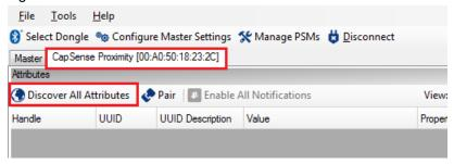
11. When all the attributes are listed, locate the Client Characteristic Configuration descriptor (UUID 0x2902) under CapSense Proximity characteristic (UUID 0x0003CAA1-0000-1000-8000-00805F9B0131). Click Read Value to read the existing CCCD value as shown in Figure 4-38.
