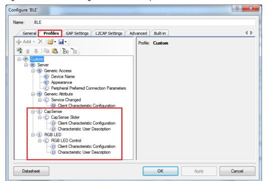
Figure 4-7. Attributes Configuration in BLE Component for Custom Services
