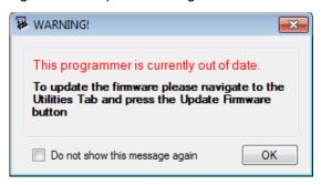
To update the KitProg, go to the **Utilities** tab on PSoC Programmer and click **Upgrade Firmware**, as shown in Figure 3-19.
