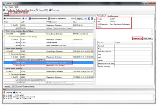
12. Modify the **Value** field of CCCD to '01:00' and click **Write Value**. This enables the notifications on the CapSense slider characteristic.
