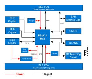
This BLE Pioneer Kit includes the PSoC 4 BLE Module. This module acts as a basic breakout board for the CY8C4248LQI-BL583 (PSoC 4 BLE) device. Besides the PSoC 4 BLE Module, there are additional modules available, which can be ordered separately. The complete list is available in BLE Modules and BLE Dongles Compatible with the BLE Pioneer Kit on page 115.
