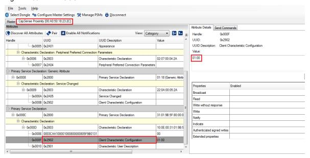
13. Bring your hand closer to the proximity sensor on the BLE Pioneer Kit, as shown in Figure 4-40 and observe the value changing in the characteristic value field, as shown in Figure 4-41.
