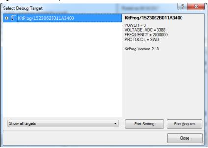
10. After the device is acquired, it is shown in a structure below the KitProg. Click the **Connect** button and then **OK** to exit the window and start programming, as shown in Figure 4-6.
