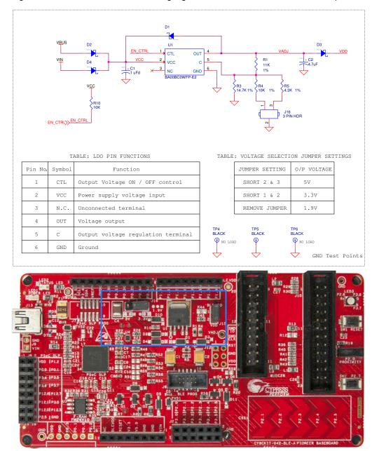
The input to the LDO can come from either the USB, the VIN pin in the Arduino header J1, or header J9.
