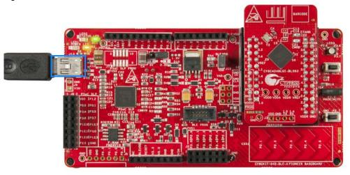
Figure 3-8. Connect Dongle to PC
