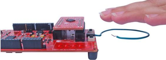
Figure 4-41. CapSense Proximity Notification Received
