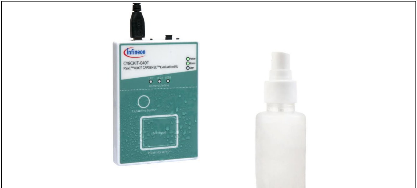
Figure 8 Water tolerance with water droplets sprayed on sensors
