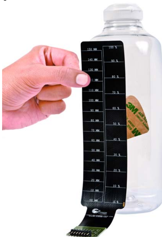
Figure 2-5. Placing the Sensor
