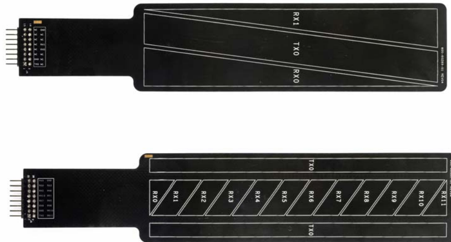
Figure 2-4. Bottom View of both CY8CKIT-022 Sensors
