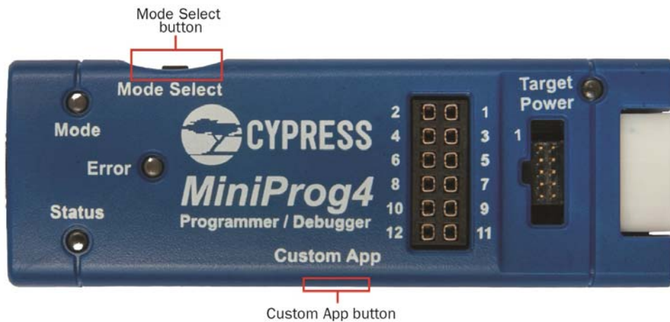
Figure 2-7. Various MiniProg4 Button Modes
