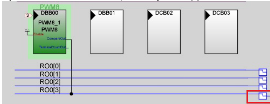
Figure 3-57. Route the PWM CompareOut signal to P0[7]
