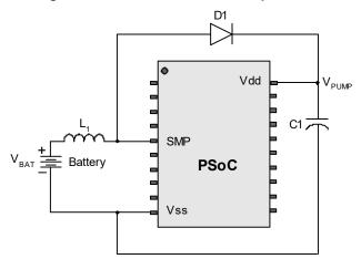
Figure 12. Basic Switch Mode Pump Circuit
