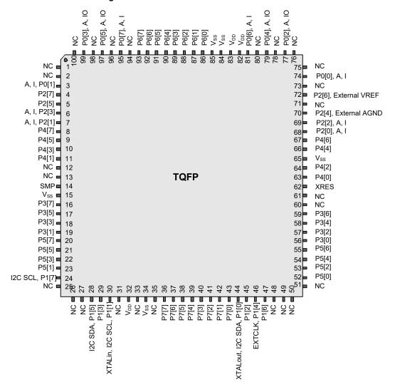
Figure 8. CY8C29866 100-Pin PSoC Device
