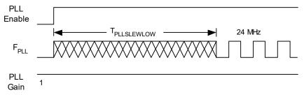
Figure 15. External Crystal Oscillator Startup Timing Diagram
