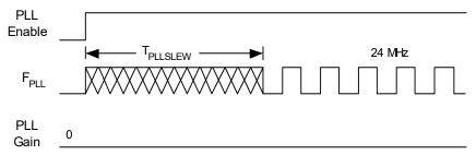
Figure 14. PLL Lock for Low Gain Setting Timing Diagram
