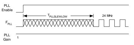
Figure 15. External Crystal Oscillator Startup Timing Diagram
