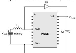
Figure 13. Basic Switch Mode Pump Circuit
