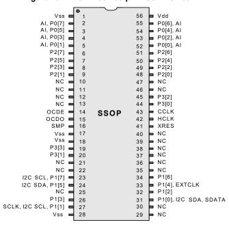
Figure 10. CY8C21001 56-pin PSoC Device
