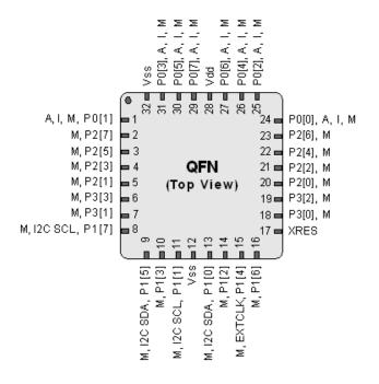
Figure 8. CY8C21634 32-pin PSoC Device
