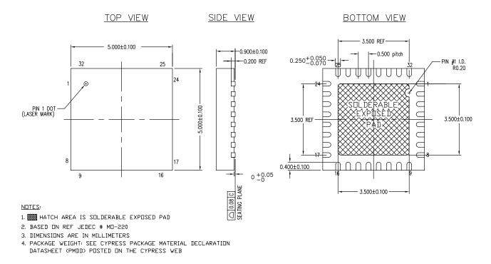
Figure 19. 32-pin QFN (5 × 5 × 1.0 mm) Package Outline, 001-30999
