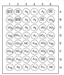
Figure 2. 48-ball VFBGA (6  $\times$  8  $\times$  1.0 mm) pinout with ERR (Top View) [4]
