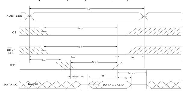
Figure 11. Write Cycle No. 3 (WE controlled) [36, 38, 39]
