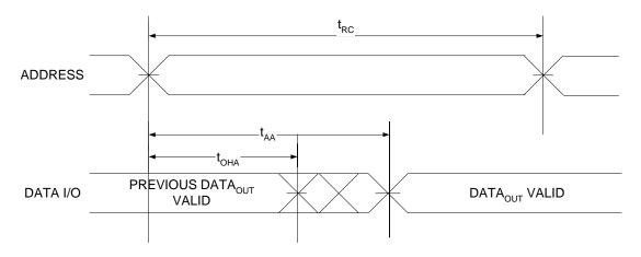
Figure 7. Read Cycle No. 2 of CY7S1061GE (Address Transition Controlled)  $^{[28,\ 29]}$
